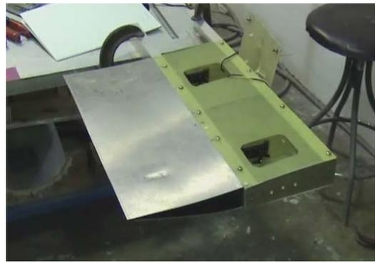
Fig. 7. Hingeless control surface with constant negative chord-wise actuation
