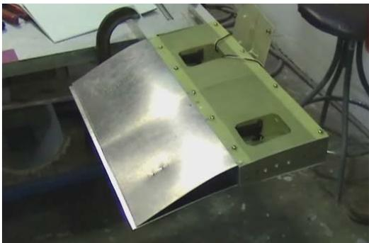
Fig. 6. Hingeless control surface with constant positive chord-wise actuation
