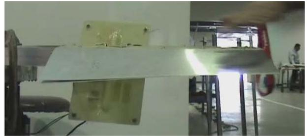
Fig. 8. Hingeless control surface with twisting actuation
