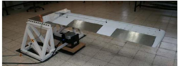
Fig. 15. The mission adaptive wing, modal shaker and accelerometers in the experimental modal analysis
