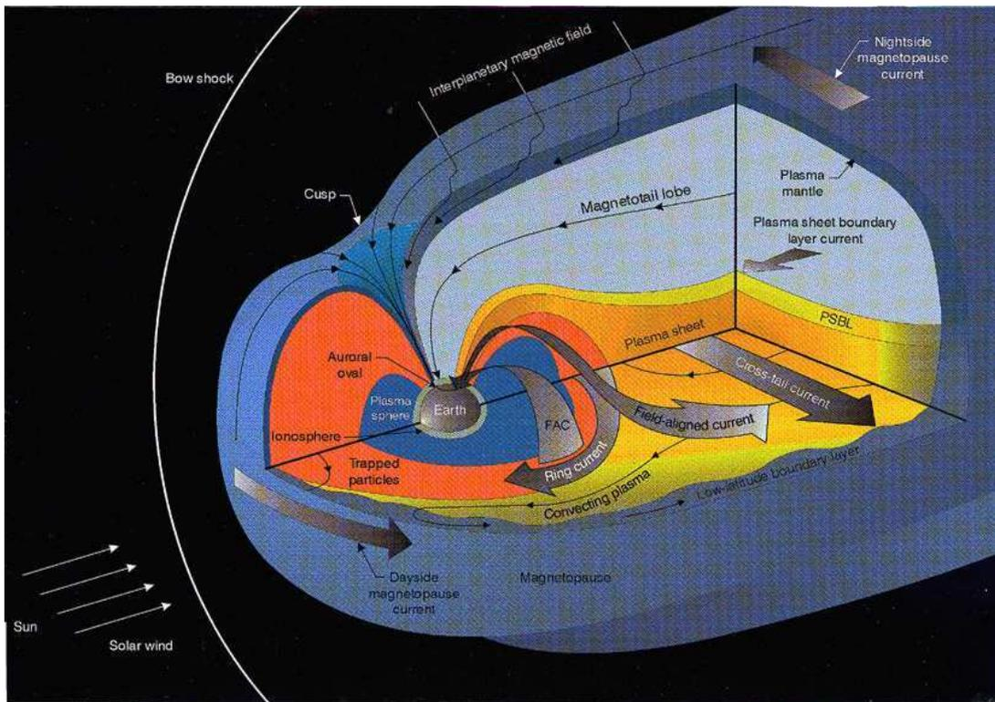
Figure 1.1: The Structure of the Magnetosphere
