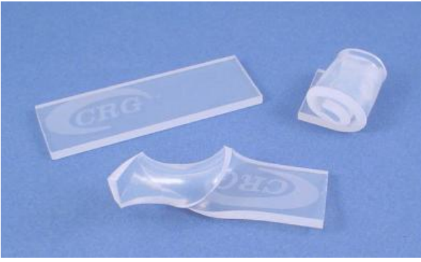
Fig. 11. A shape memory polymer used for morphing air vehicle applications [26].
