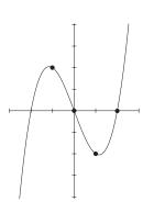
Typically the interface would allow the user to enter control points by clicking them in with the mouse. For example, say the user has entered control points (-1,2),(0,0),(1,-2),(2,0) as indicated by the dots in the figure to the left.
