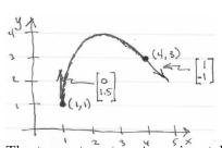
In the example to the left,  $\mathbf{p}_i = (1,1)$ , and  $\mathbf{p}_{i+1} = (4,3)$ , thus  $\frac{du_i}{dx} = \frac{1-0}{4-1} = \frac{1}{3}$ , and  $\frac{du_i}{dy} = \frac{1-0}{3-1} = \frac{1}{2}$ . The tangent vectors are  $\mathbf{t}_i = \begin{bmatrix} 0 \\ 1.5 \end{bmatrix}$ , and  $\mathbf{t}_{i+1} = \begin{bmatrix} 1 \\ -1 \end{bmatrix}$ .
