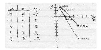
We see that the curve is described in 2-dimensional space, and unlike the graph of a function it can wrap back on itself. By picking appropriate functions x = f(u) and y = g(u) we can describe whatever 2D shape we desire.
