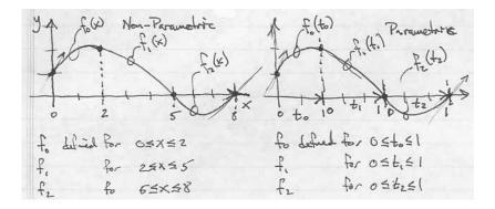
In the example, both curves are identical, however, the equations describing them will be different. In the parametric form on the right, we have defined parameters  $t_0$ ,  $t_1$  and  $t_2$  that vary between 0 and 1 as we step along the x axis between control points. We could write equations:
