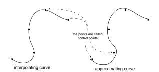
Once we establish this interface, then to change the shape of the curve we just move the control points.
