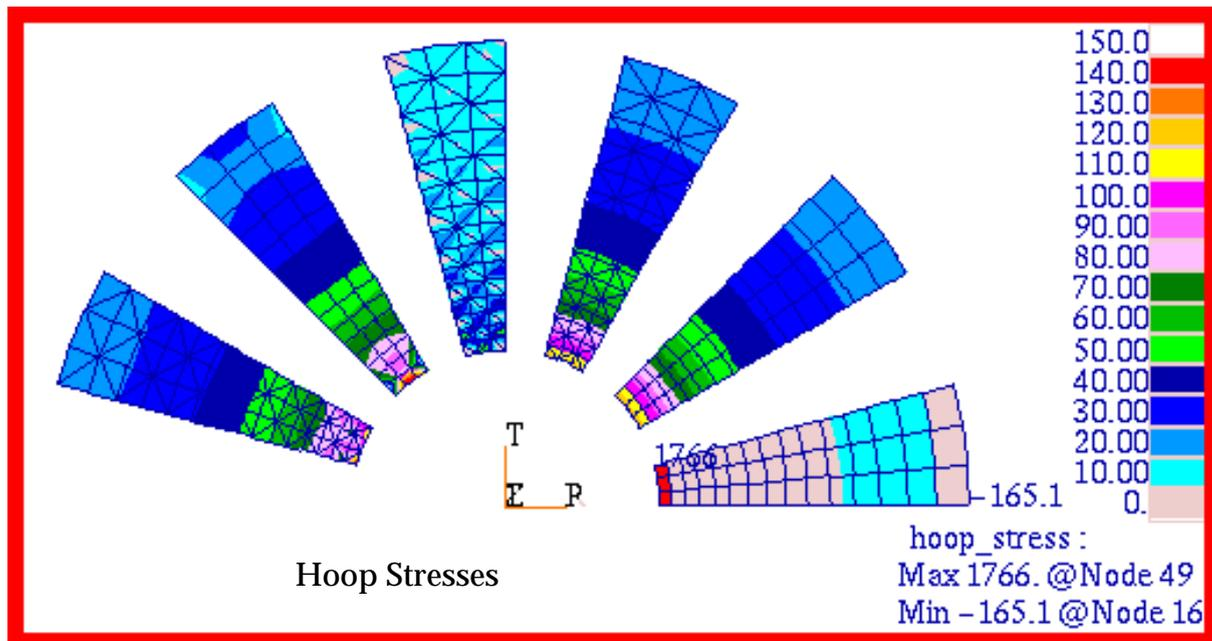
Figure 15-31 Fringe Plot of Hoop Stress,  $\sigma_\theta$ , on 2D Solid Elements.
