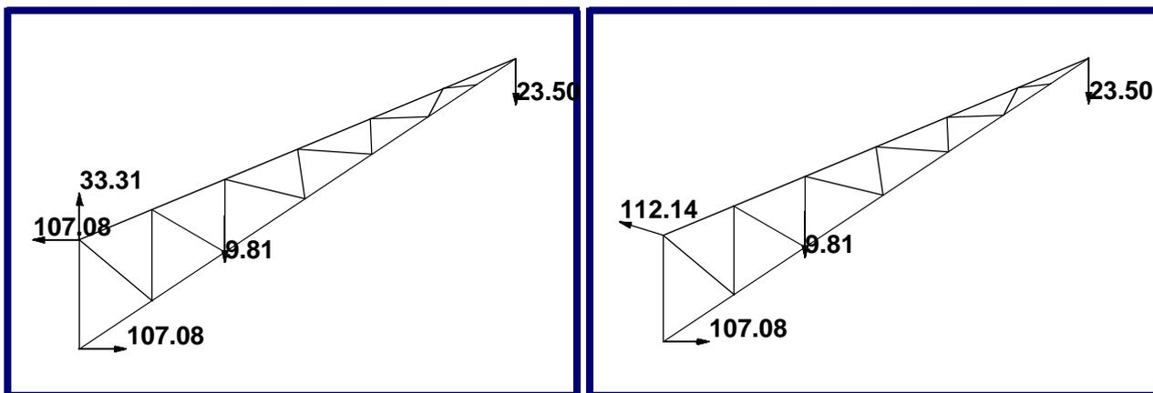
**Figure 12-3 Example Plot of the Total Freebody Diagram for the Continuous Truss Example. Both Resultant and Component Displays are Shown.**
