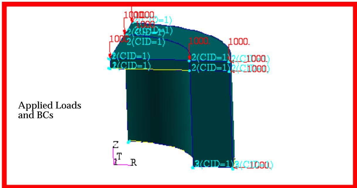
Figure 15-49 Loads and Boundary Conditions of Cylinder.
