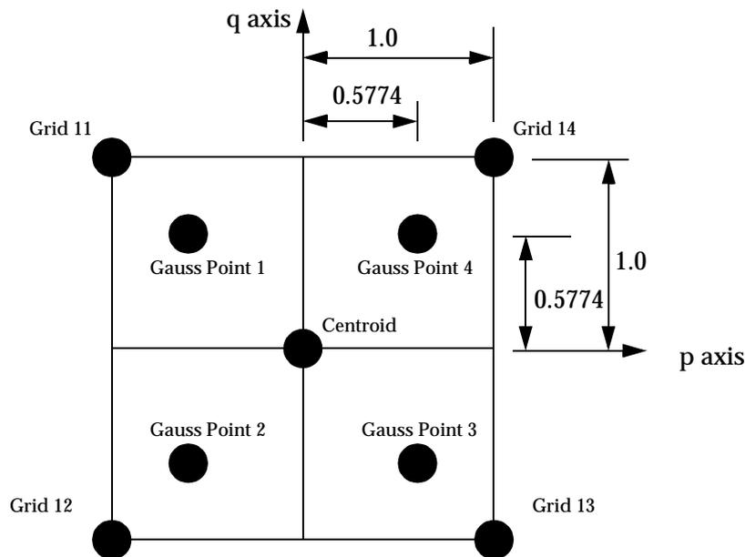
**Figure 14-3 Example 4 Noded QUAD with Gauss Points.**
