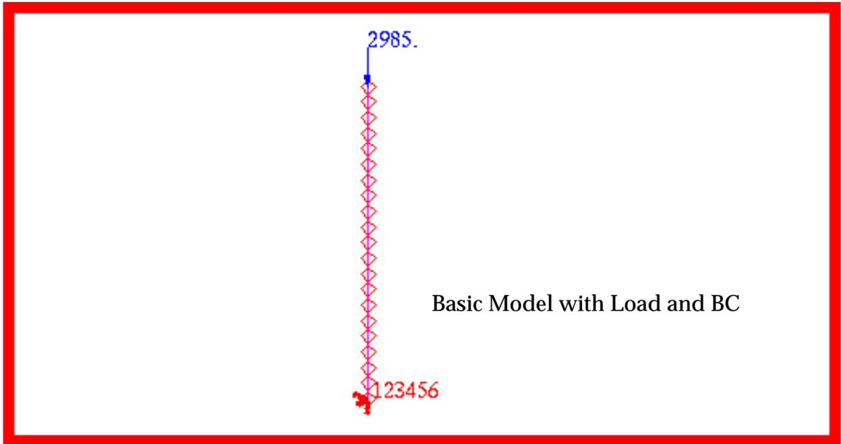
**Figure 15-83 Nonlinear Beam Post-Buckling Model.**
