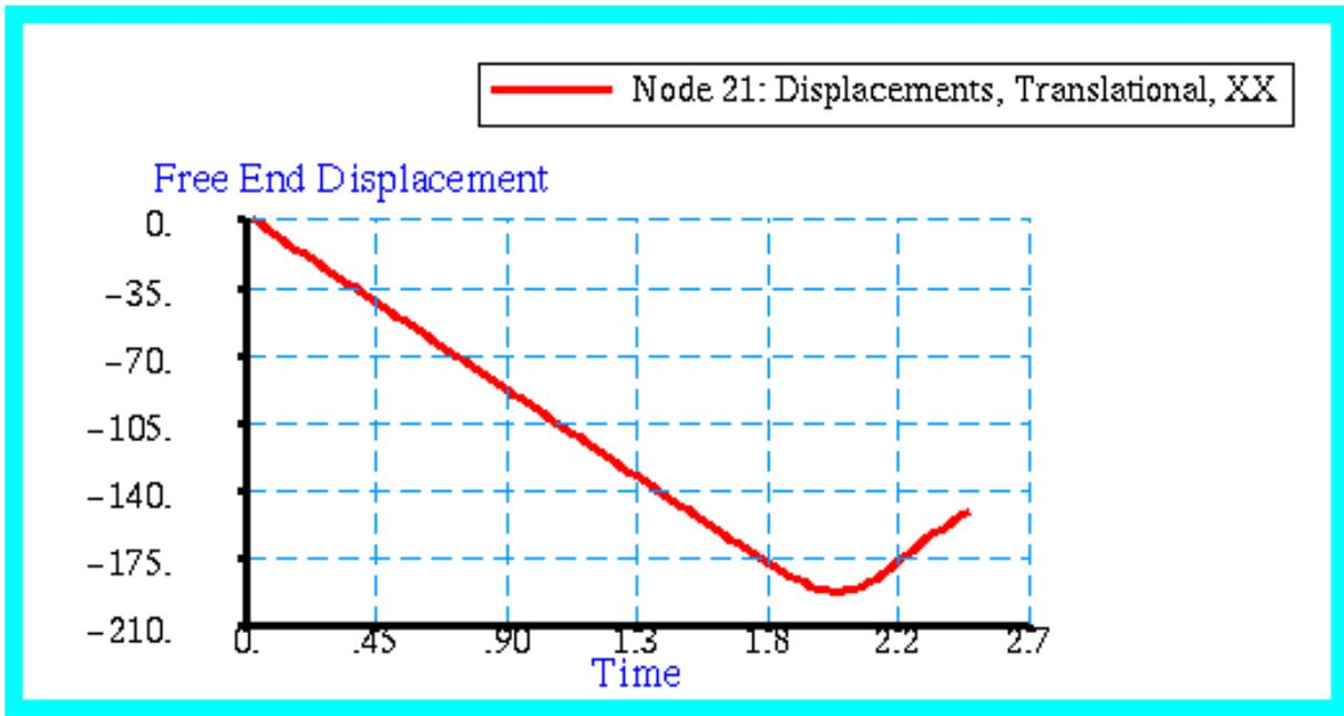
Figure 15-39 Free End Displacement of CROD Model.
