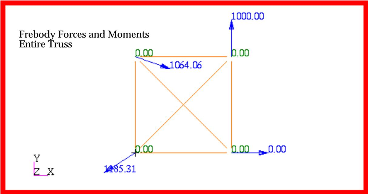
Figure 15-73 Freebody Forces and Moments for Entire Truss.
