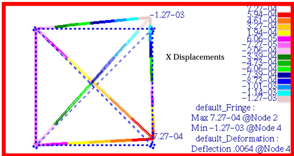
Figure 15-56 X Translational Displacement of Pinned Truss.
