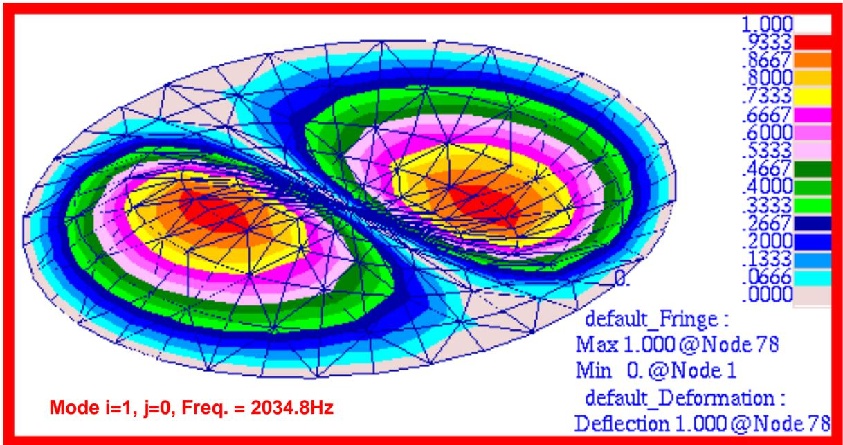
Figure 15-10 Mode 2,  $f_{10}$ , for Membrane h-Element Model.
