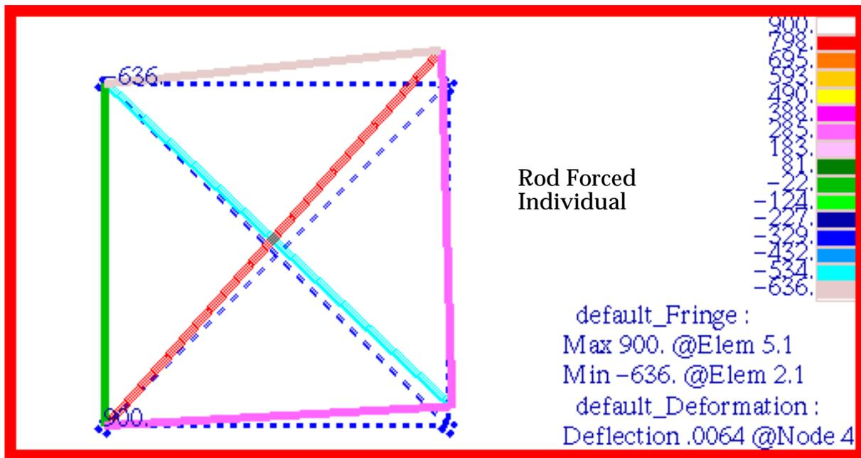
Figure 15-58 Rod Forces from Pinned Truss Analysis.
