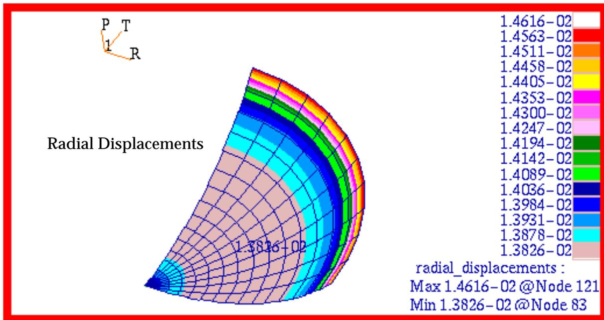
Figure 15-33 Radial Displacement of Spherical Membrane.
