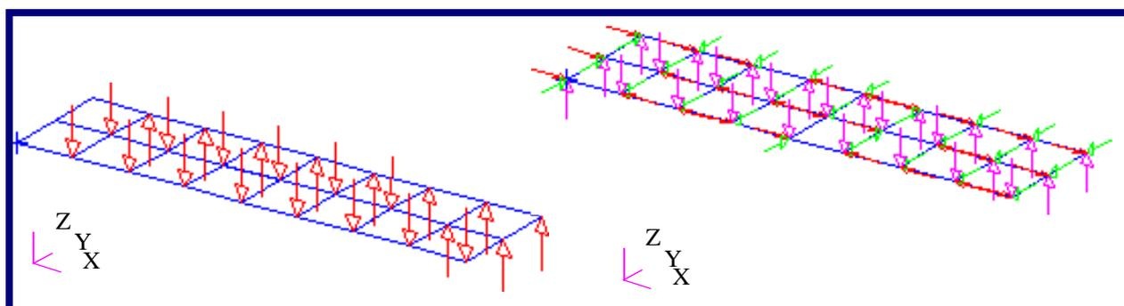
**Figure 6-1 Resultant and Component Vector Plots of Displacement on Cantilever Plate (constant vector lengths).**
