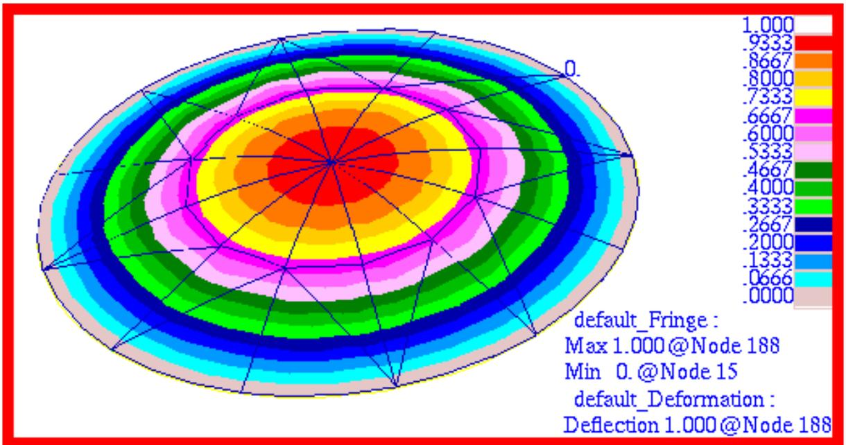
Figure 15-16 Mode 1,  $f_{00}$ , of p-Element Membrane Model.
