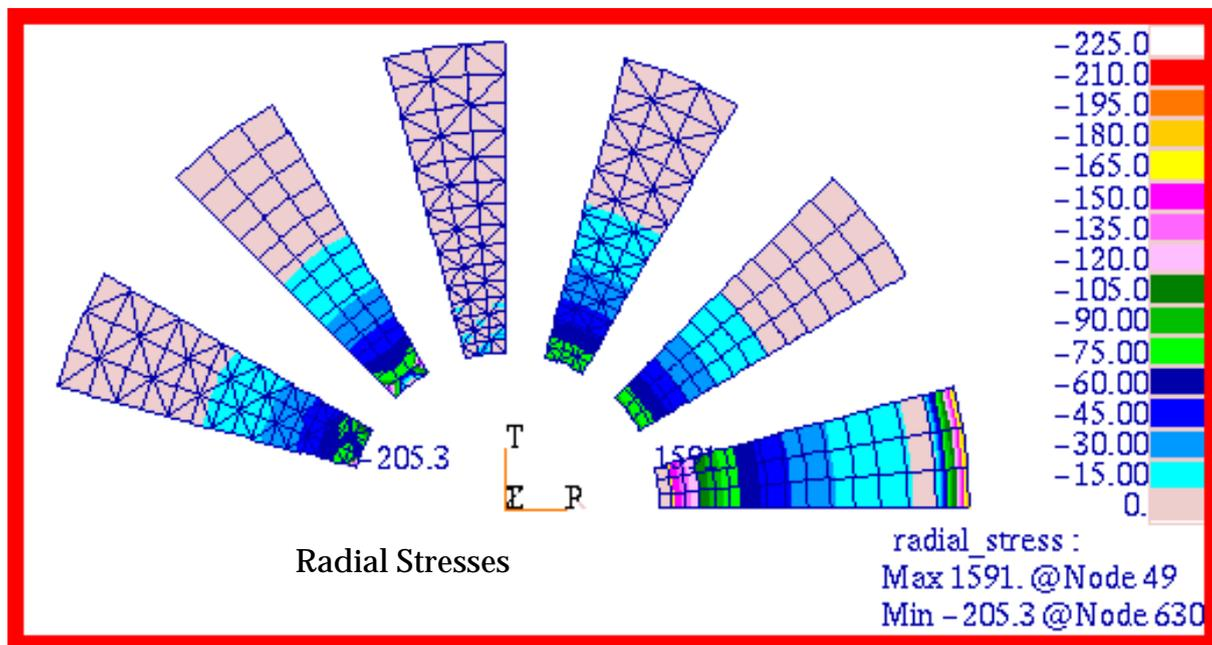
Figure 15-30 Fringe Plot of Radial Stress,  $\sigma_r$ , on 2D Solid Elements.
