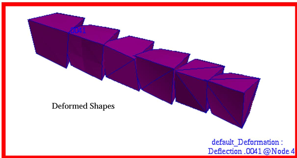
Figure 15-66 Deformed Shape of Elements Due to Thermal Gradient.
