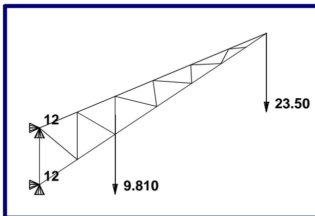
**Figure 12-1 Example Plot of Applied Loads for the Continuous Truss Example**
