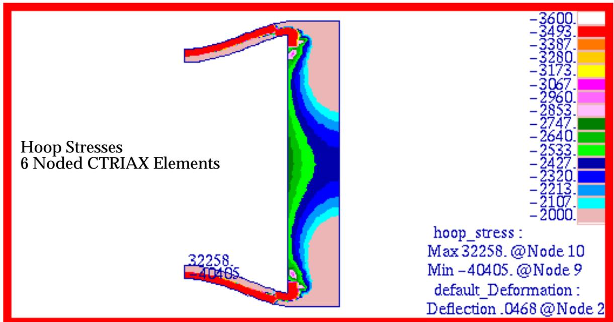
Figure 15-44 Hoop Stress in 6 Noded Axisymmetric Model.
