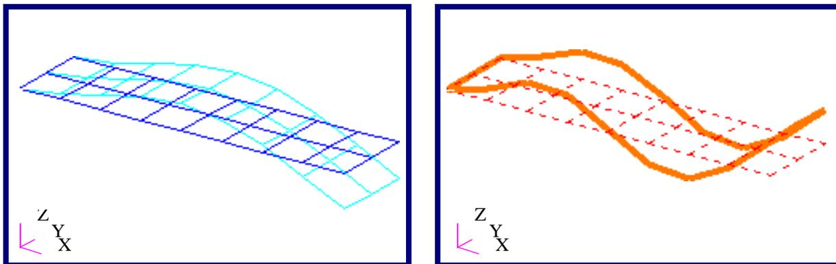
**Figure 3-6 Two Deformation Plots in Separate Viewports, 2nd Bending Model in Wireframe and 3rd Bending in Free Edge Display.**
