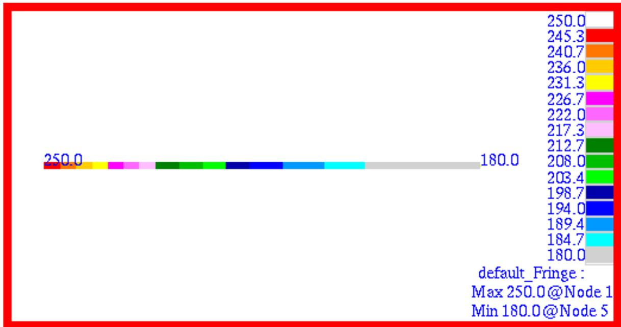
Figure 15-65 Nodal Temperatures of Cooling Fin.
