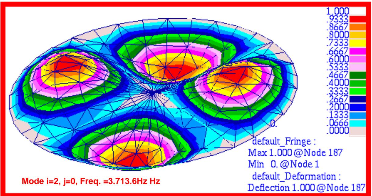
Figure 15-11 Mode 4,  $f_{20}$ , for Membrane h-Element Model.
