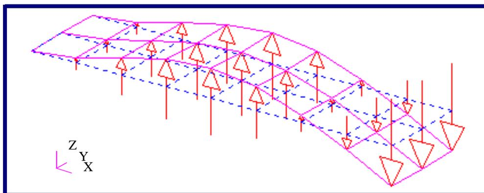
Figure 6-3 Vector Plot on a Deformed Shape (scaled vector lengths).
