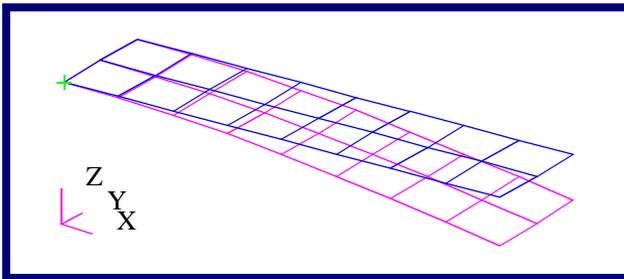
Figure 3-1 Deformation Plot of Cantilever Plate with Undeformed Shape.
