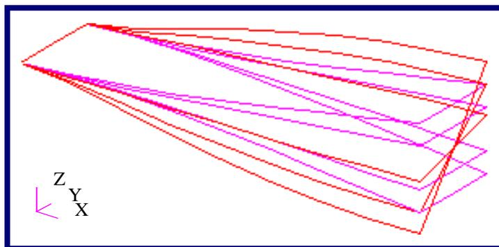
**Figure 9-2 Simultaneous Animation of a Bending Mode (Magenta) and a Torsional Mode (Red).**
