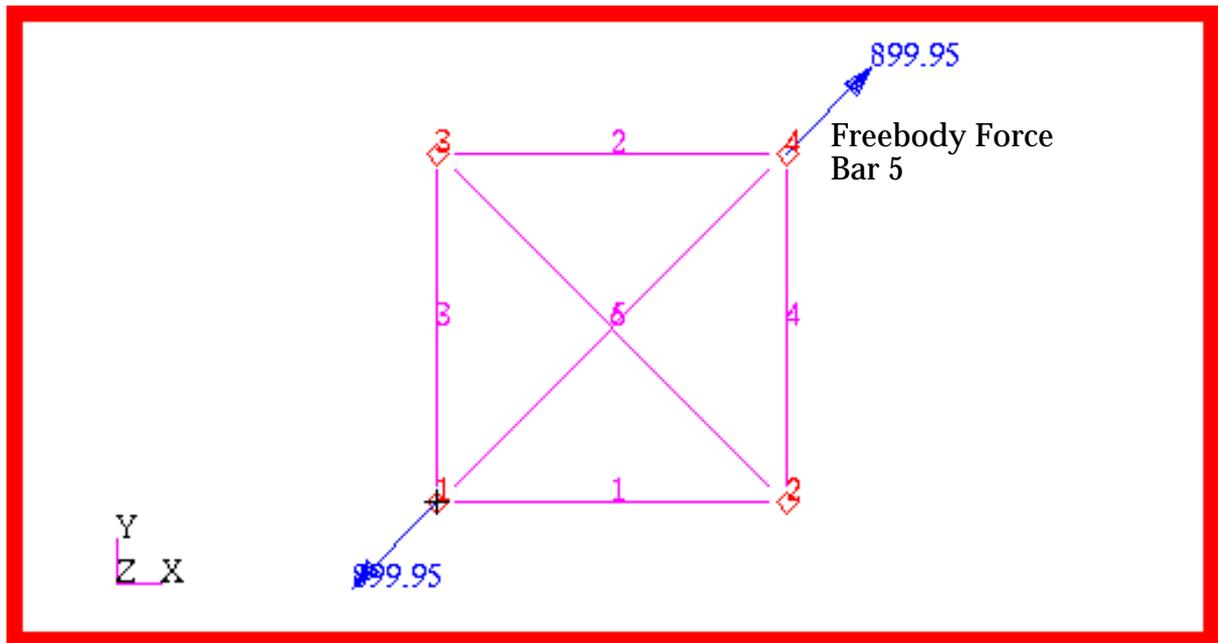
Figure 15-71 Freebody Forces in Bar 5.
