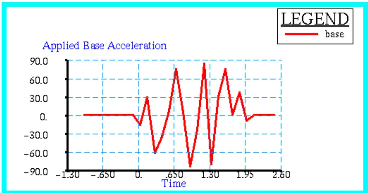
Figure 15-30 Horizontal Acceleration Applied to Truss.
