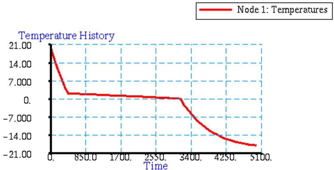
Figure 15-62 Temperature Response of Freezing Cube.
