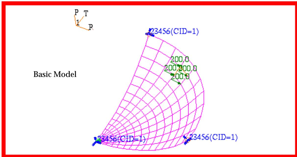
Figure 15-32 Basic Model of 2D Shell in Spherical Coordinates.
