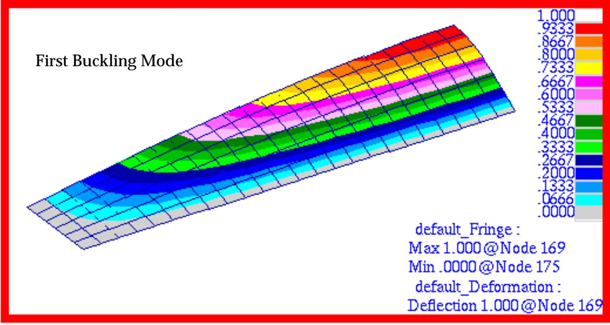
Figure 15-25 Buckling Mode Shape of Plate due to Critical Pressure.
