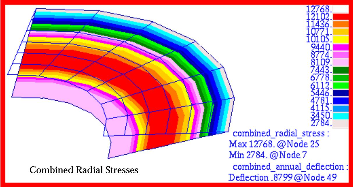
Figure 15-81 Combined Radial Stress of Annular Plate.
