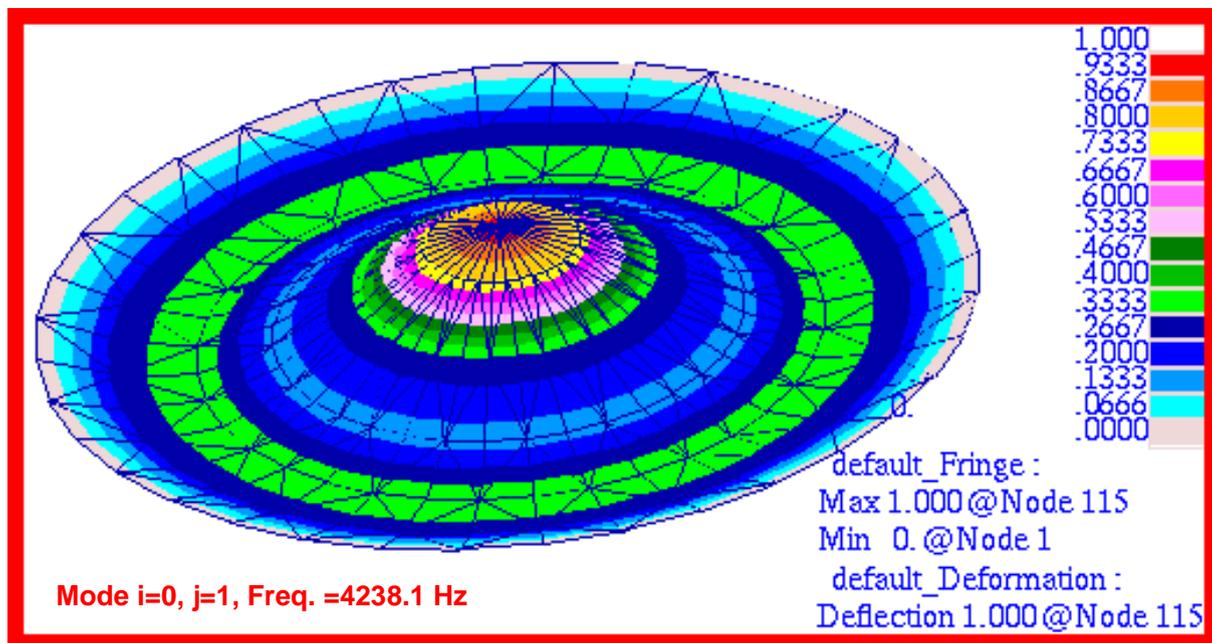
Figure 15-12 Mode 6,  $f_{01}$ , for Membrane h-Element Model.
