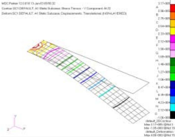
**Figure 5-2** Contour Plot of the Y-Component of Stress on Deformed Cantilever Plate.
