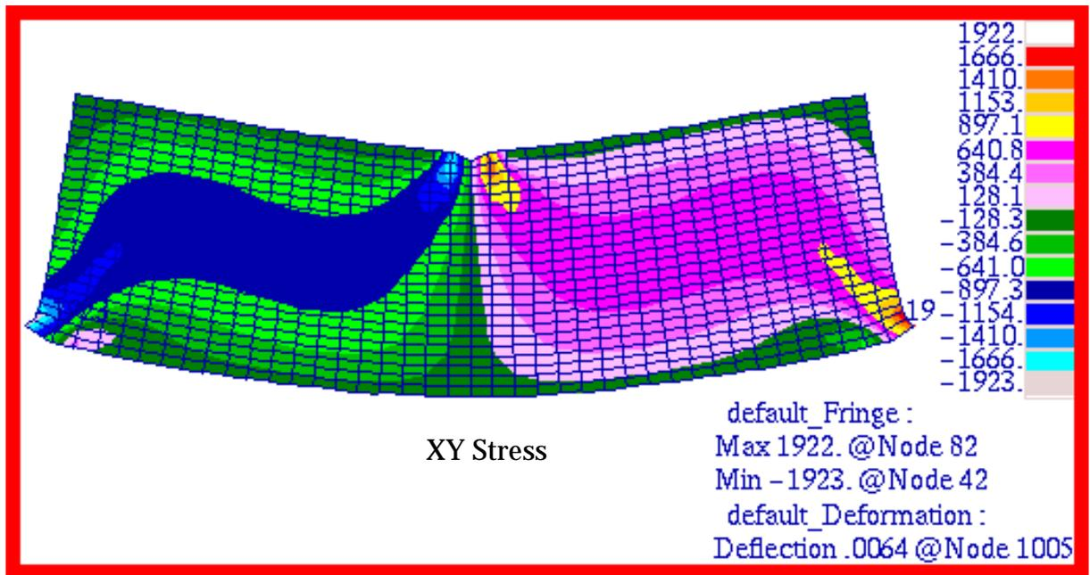
Figure 15-20  $\tau_{xy}$  Stress of Beam Model.
