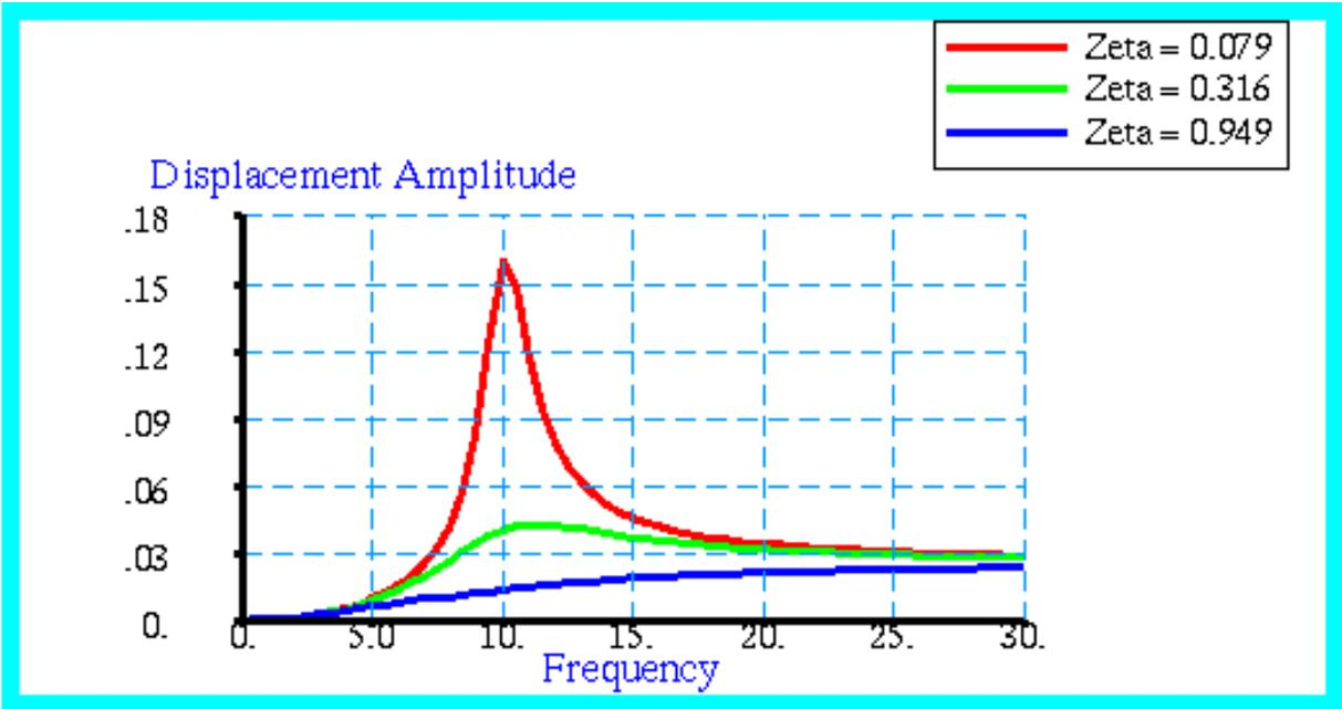
Figure 15-45 Amplitude Displacements at Center of Rod.
