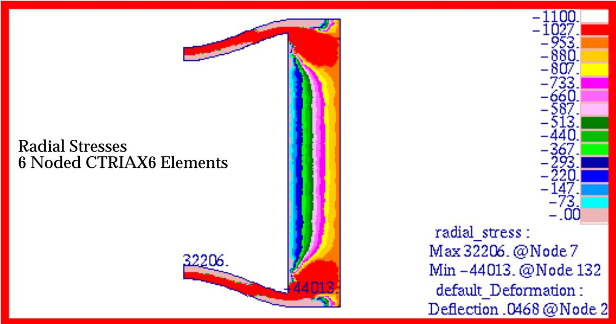
Figure 15-42 Radial Stress in 6 Noded Axisymmetric Model.
