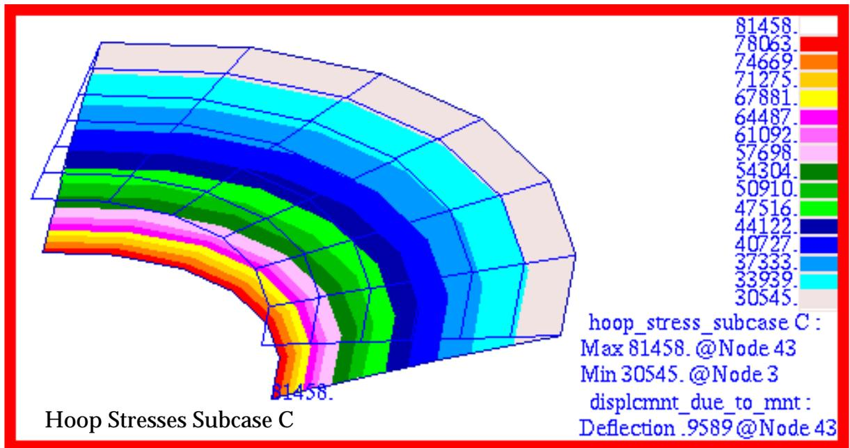
Figure 15-79 Hoop Stress of Annular Plate (Subcase C).
