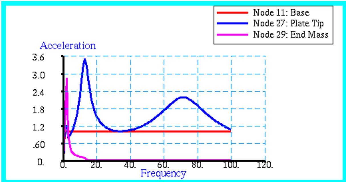
Figure 15-52 Acceleration Responses of Plate Tip, End Mass, and Base.
