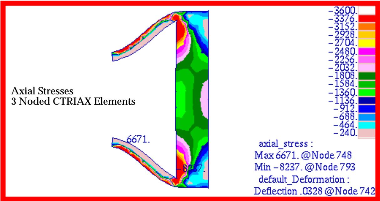
Figure 15-47 Axial Stress in 3 Noded Axisymmetric Model.
