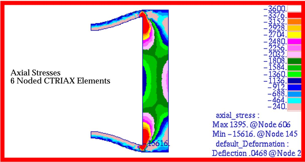
Figure 15-46 Axial Stress in 6 Noded Axisymmetric Model.
