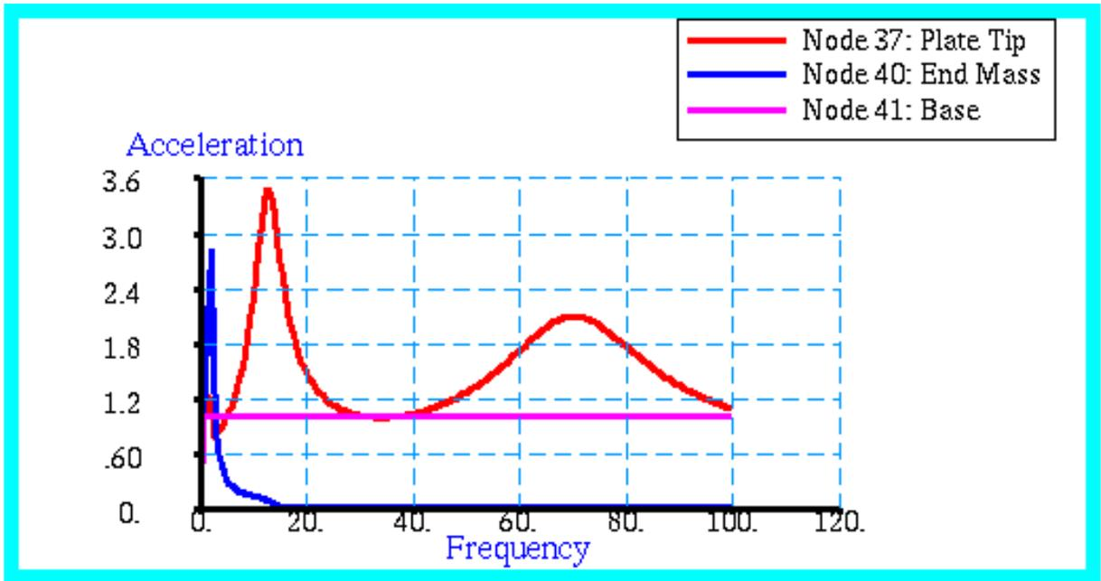
Figure 15-50 Acceleration Responses of Plate Tip, End Mass, and Base.
