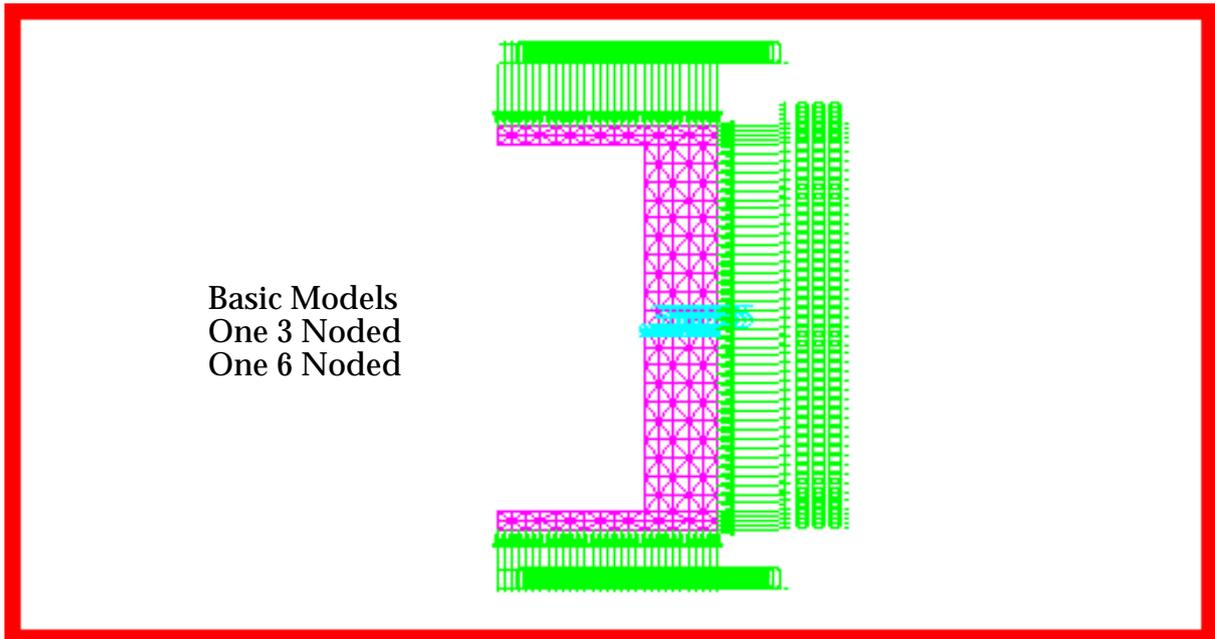
Figure 15-39 Axisymmetric Models of Thick Walled Cylinder.
