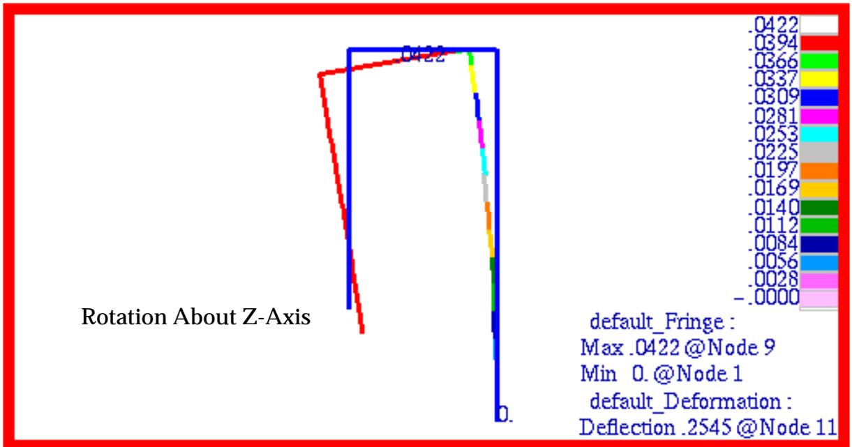
Figure 15-6 Rotational Displacement about Z-axis of Rigid Frame.
