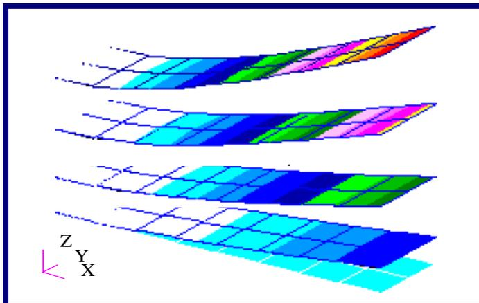
**Figure 4-3 Exaggerated Transient Animation of Displacements with Fringe Superimposed on Deformed Shape.**
