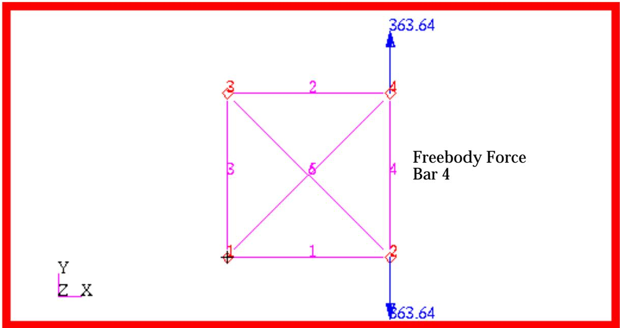
Figure 15-70 Freebody Forces in Bar 4.
