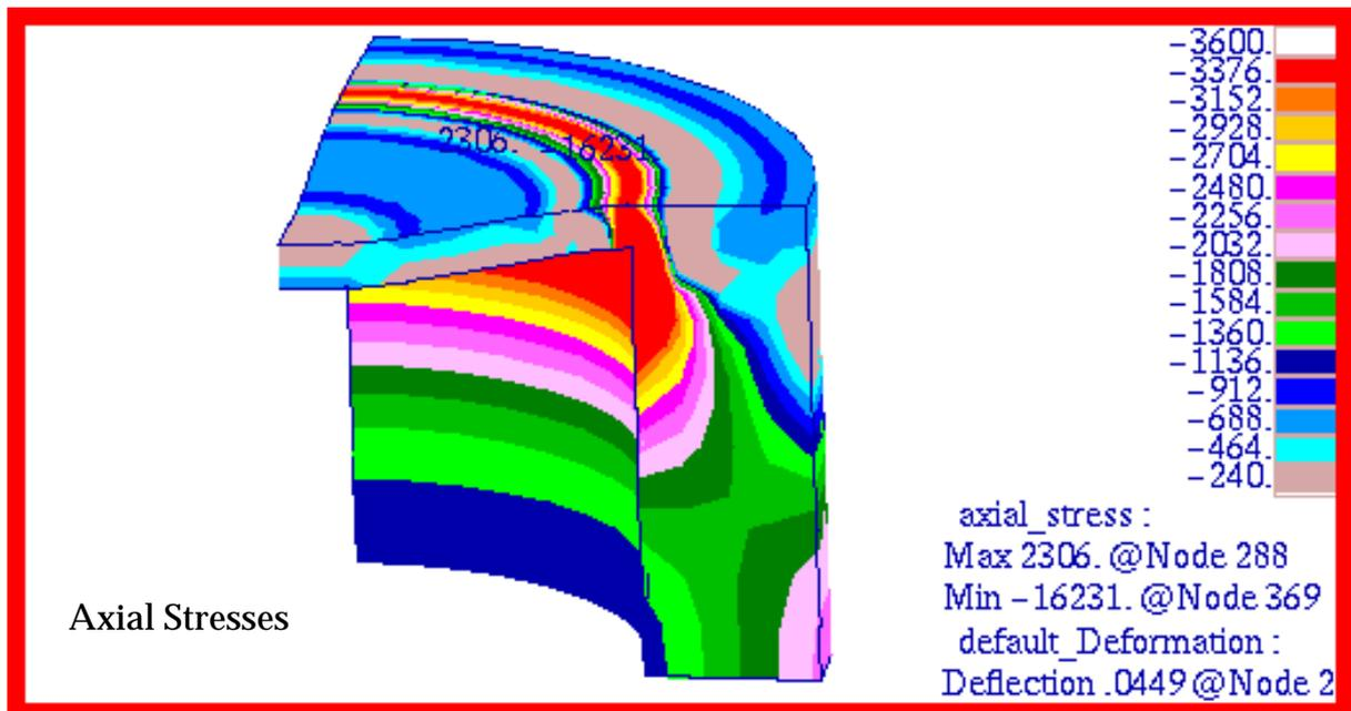
Figure 15-54 Axial,  $\sigma_1$ , Stress of Thick Walled Cylinder.
