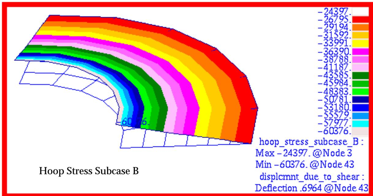
Figure 15-76 Hoop Stress of Annular Plate (Subcase B).
