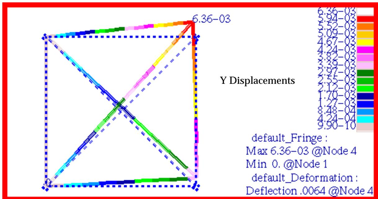
Figure 15-57 Y Translational Displacement of Pinned Truss.
