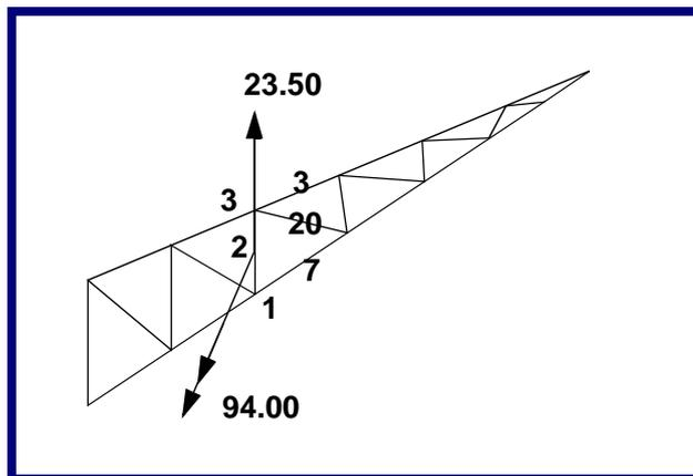
**Figure 12-5 Example Plot of Applied Loads for the Continuous Truss Example**
