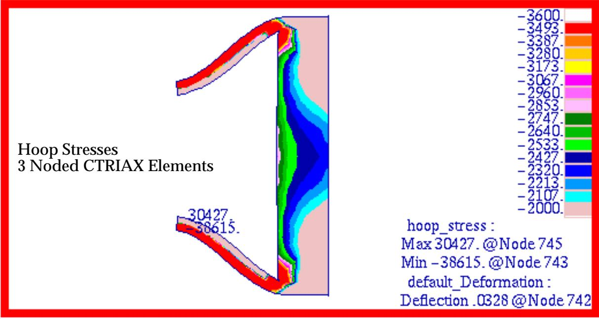
Figure 15-45 Hoop Stress in 3 Noded Axisymmetric Model.
