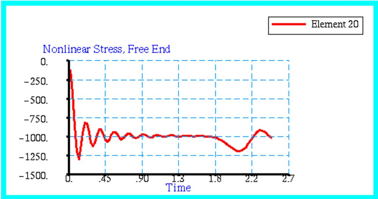
Figure 15-37 Stress History Plot at Element 20, the Free End.
