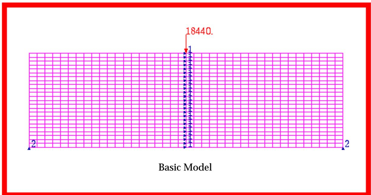
Figure 15-17 Basic Beam Model with Loads and Boundary Conditions.
