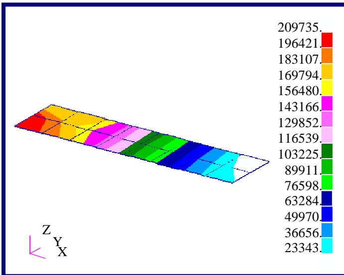
Figure 2-1 Fringe Plot of Stresses in a Cantilever Plate.
