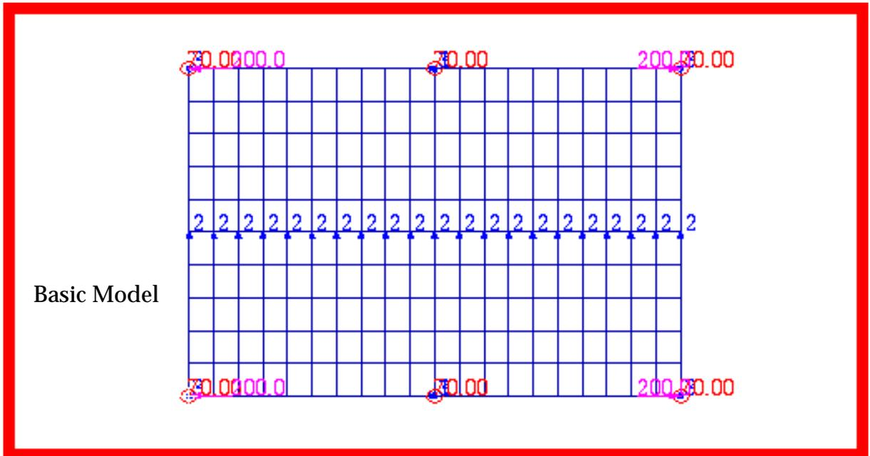
**Figure 15-7 Basic Cross-Ply FE Composite Plate Model.**
