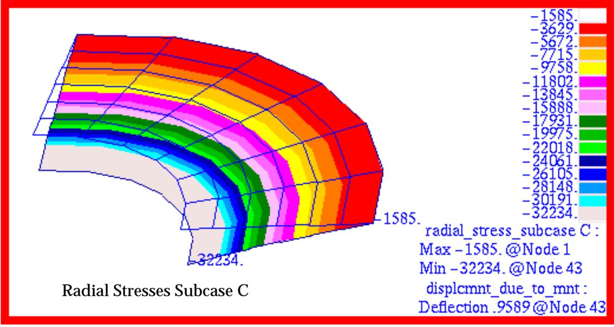
Figure 15-78 Radial Stress of Annular Plate (Subcase C).
