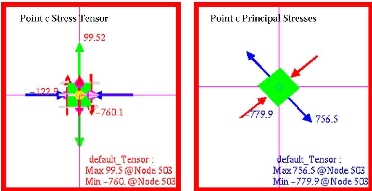
Figure 15-26 Stress Tensor and Principal Stresses at Point c.
