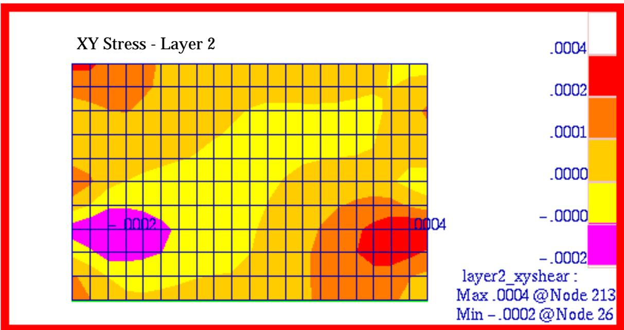
Figure 15-13 Cross-Ply Composite Plate,  $\tau_{xy}$  Stress, Layer 2.
