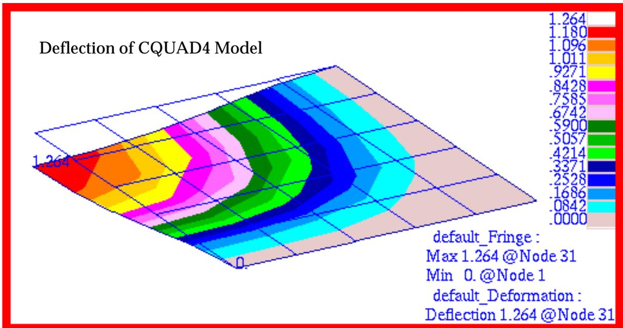
Figure 15-62 Large Deflection Displacements of CQUAD4 Model.
