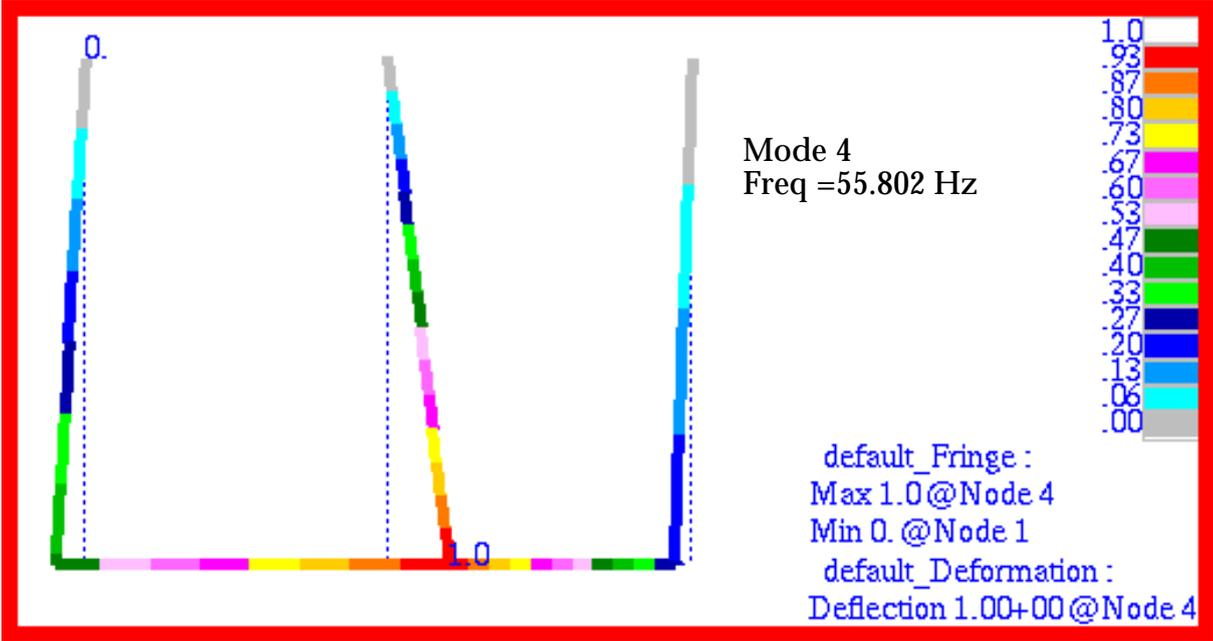
Figure 15-57 Complex Mode 4 of Pendulums, Freq = 55.802 Hz.
