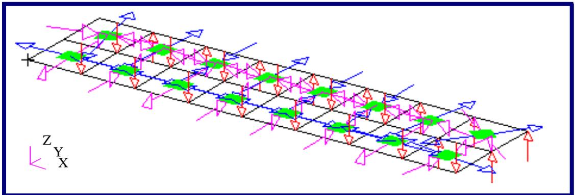
Figure 6-2 Principal Tensor Plot of Stresses on Cantilever Plate (constant vector lengths).
