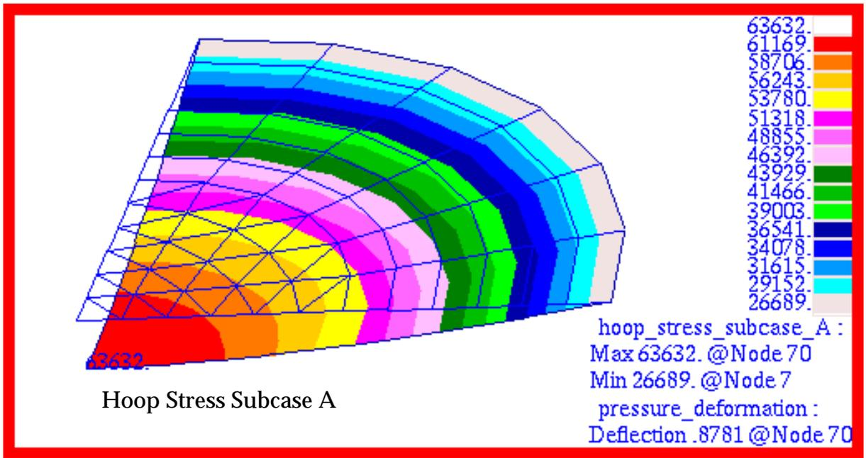
Figure 15-73 Hoop Stress of Circular Plate (Subcase A).
