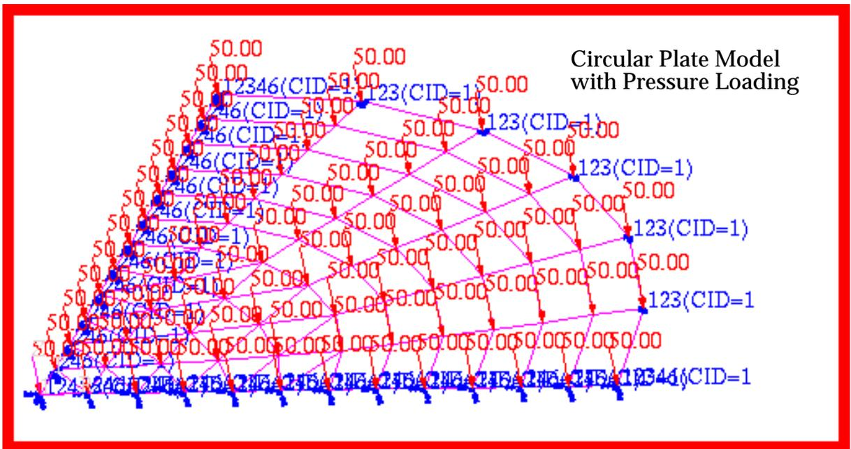
Figure 15-68 Model of Pressurized Circular Plate (Subcase A).
