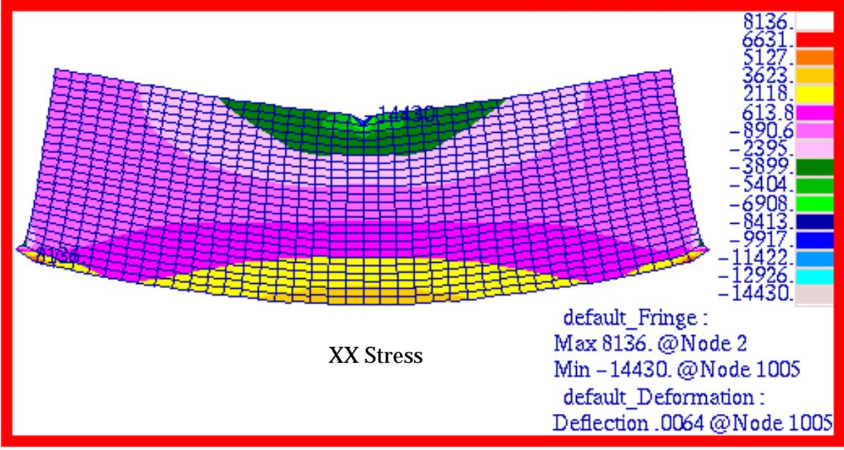
Figure 15-18  $\sigma_x$  Stress of Beam Model.
