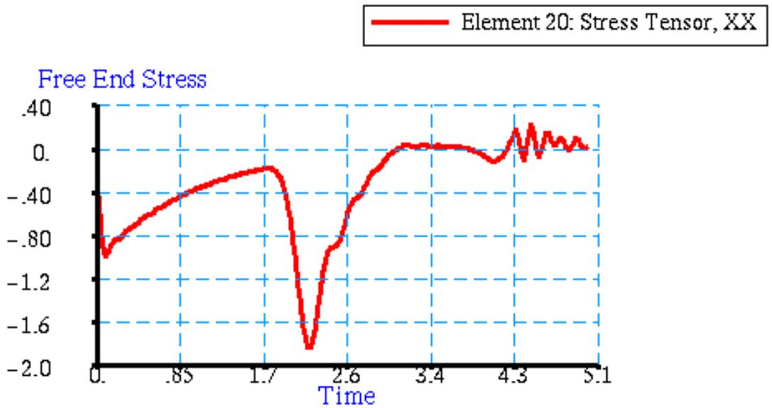
Figure 15-41 Free End Stress Response of Impact Model.
