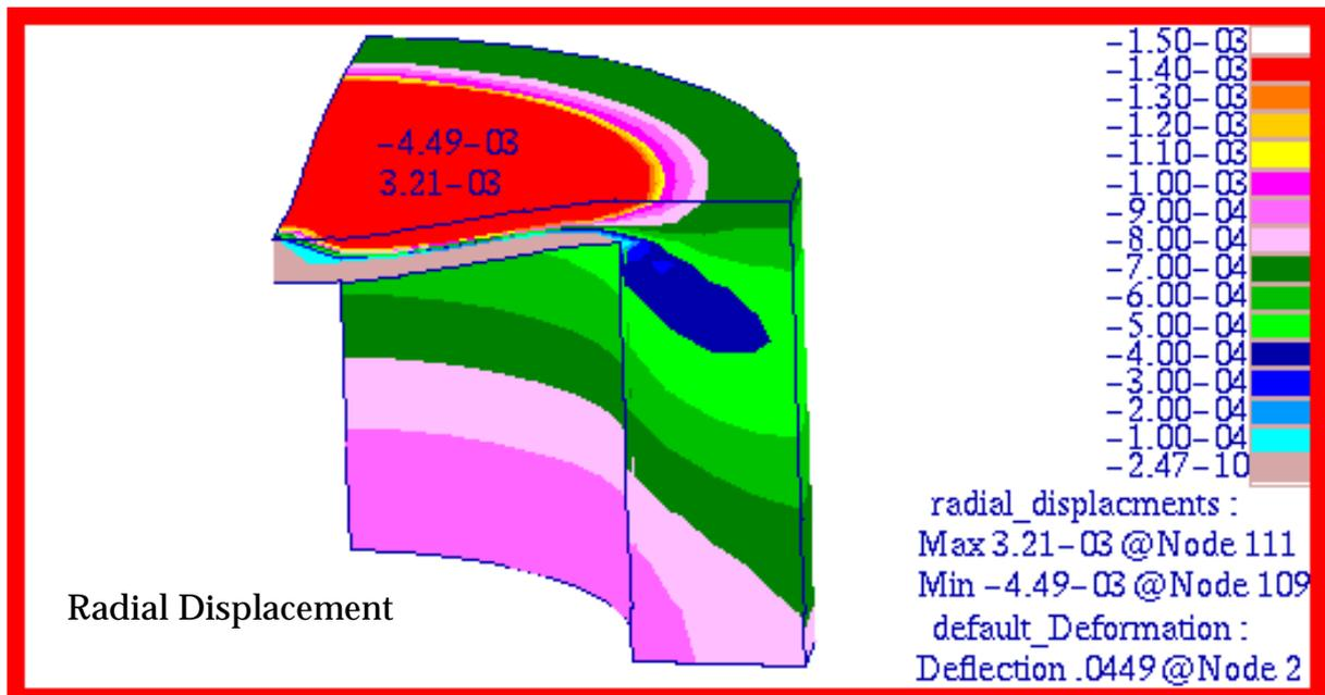
Figure 15-50 Radial Displacements of Thick Walled Cylinder.
