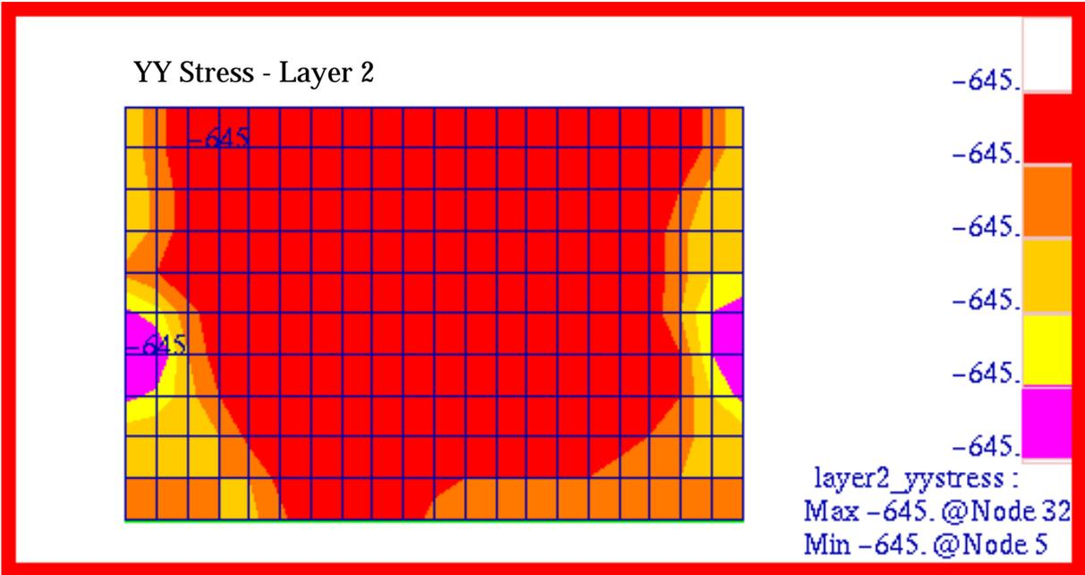
Figure 15-12 Cross-Ply Composite Plate,  $\sigma_y$  Stress, Layer 2.
