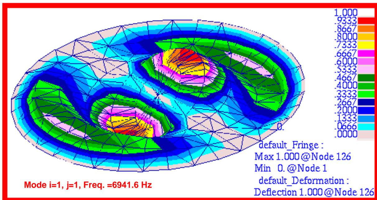
Figure 15-13 Mode 9,  $f_{11}$ , for Membrane h-Element Model.
