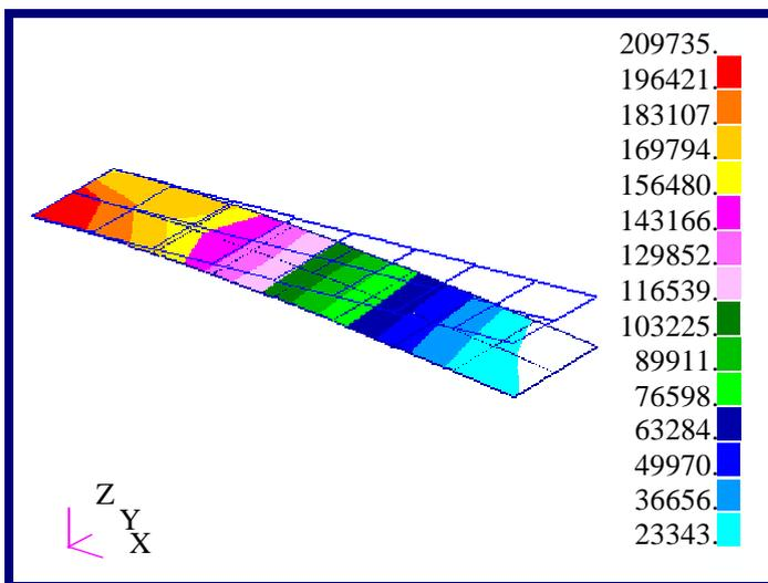
**Figure 4-2 Fringe Plot of von Mises Stress on Deformed Cantilever Plate.**
