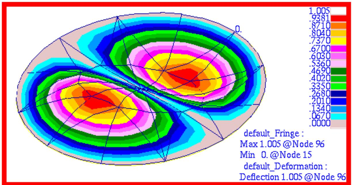
Figure 15-17 Mode 2,  $f_{10}$ , of p-Element Membrane Model.
