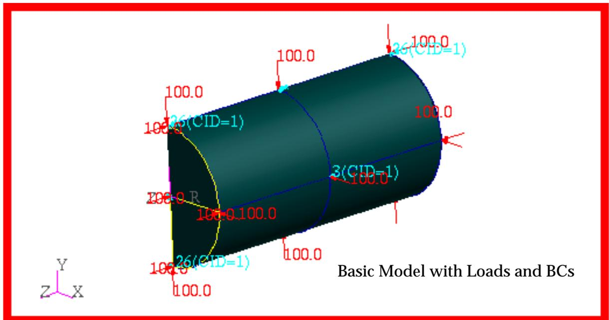
**Figure 15-22 Cylinder Buckling Model with Loads and BCs.**
