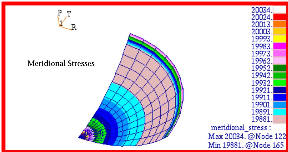
Figure 15-37 Meridional Stresses of Spherical Membrane.
