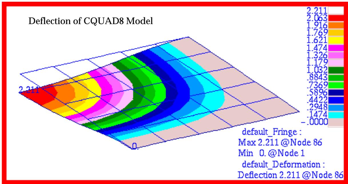
Figure 15-63 Large Deflection Displacements of CQUAD8 Model.
