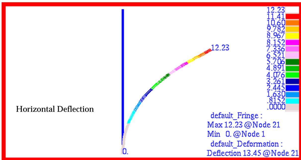
Figure 15-84 Post-Buckled Horizontal Deformation of Beam.
