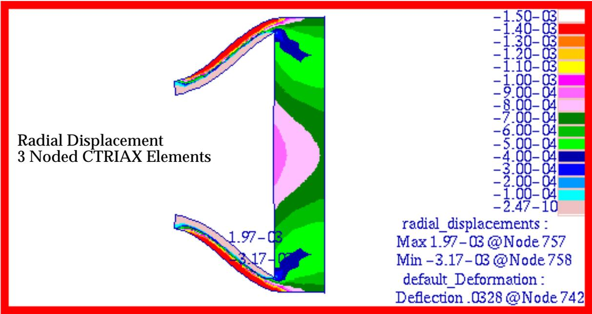
Figure 15-41 Radial Displacement of 3 Noded Axisymmetric Model.
