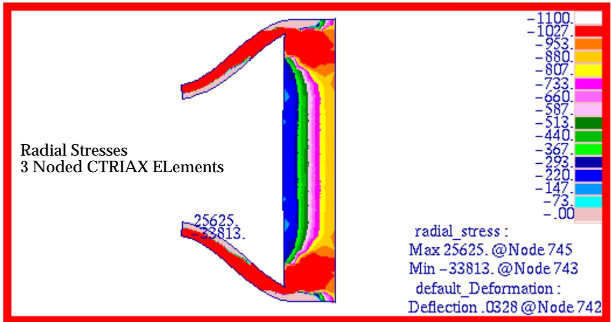
Figure 15-43 Radial Stress in 3 Noded Axisymmetric Model.
