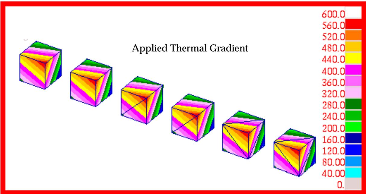
Figure 15-65 Thermal Gradient Applied to Solid Elements.
