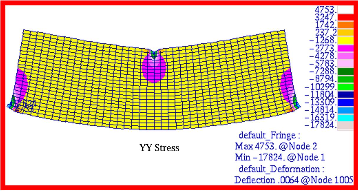
Figure 15-19  $\sigma_y$  Stress of Beam Model.
