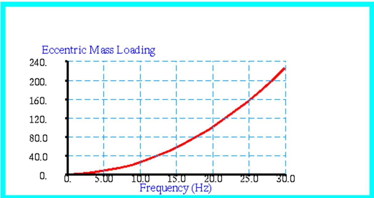
Figure 15-44 Applied Force versus Frequency.
