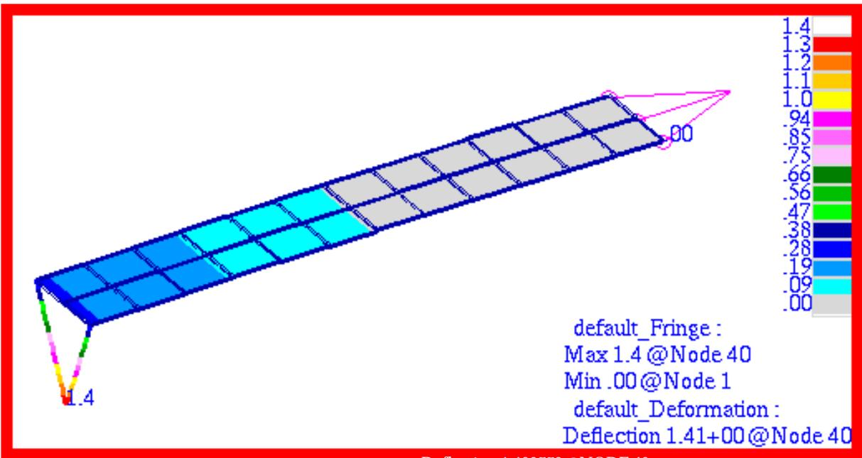
Figure 15-47 First Mode Shape of Beam, Freq=2.0054 Hz.
