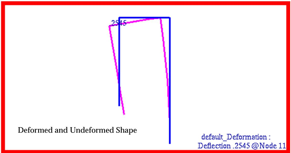
Figure 15-2 Deformed and Undeformed Shape of Rigid Frame.
