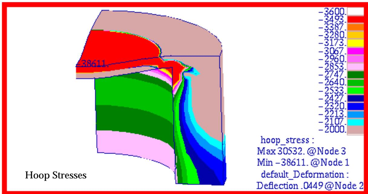
Figure 15-53 Hoop,  $\sigma_2$ , Stress of Thick Walled Cylinder.
