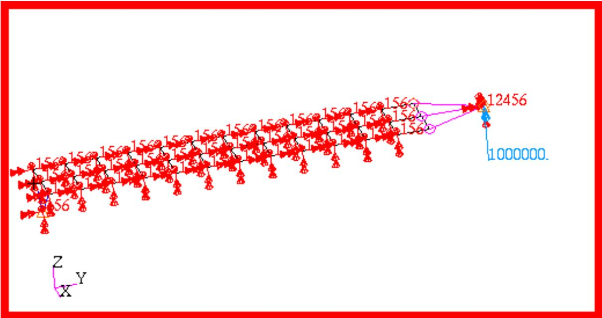
Figure 15-46 Model of Beam with Suspended Mass.
