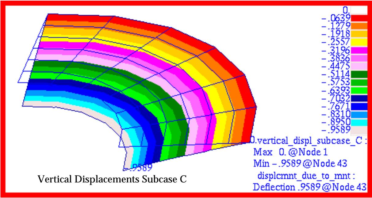
Figure 15-77 Vertical Displacement of Annular Plate (Subcase C).
