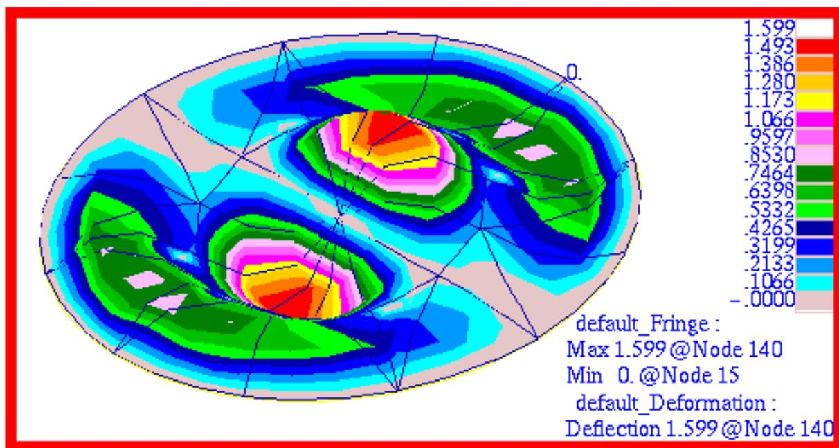
Figure 15-20 Mode 9,  $f_{11}$ , for Membrane p-Element Model.
