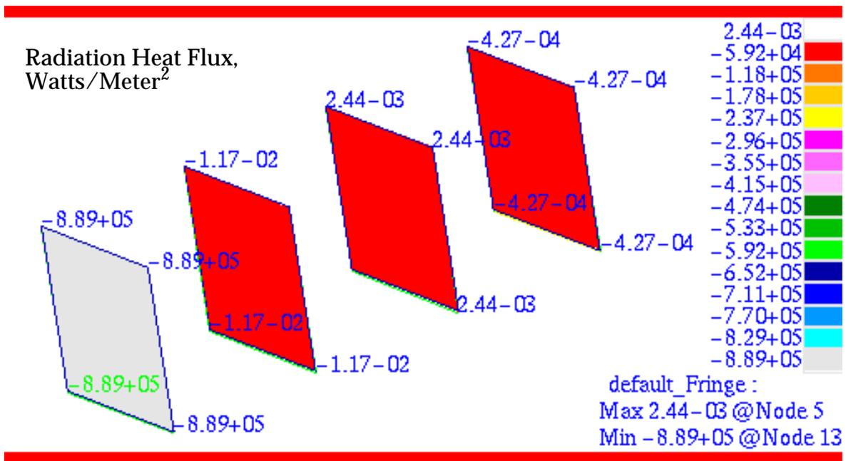
Figure 15-60 Radiation Heat Fluxes of the Four Parallel Plate.
