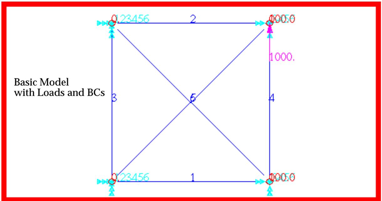
Figure 15-55 Basic Pinned Truss Analysis Model.
