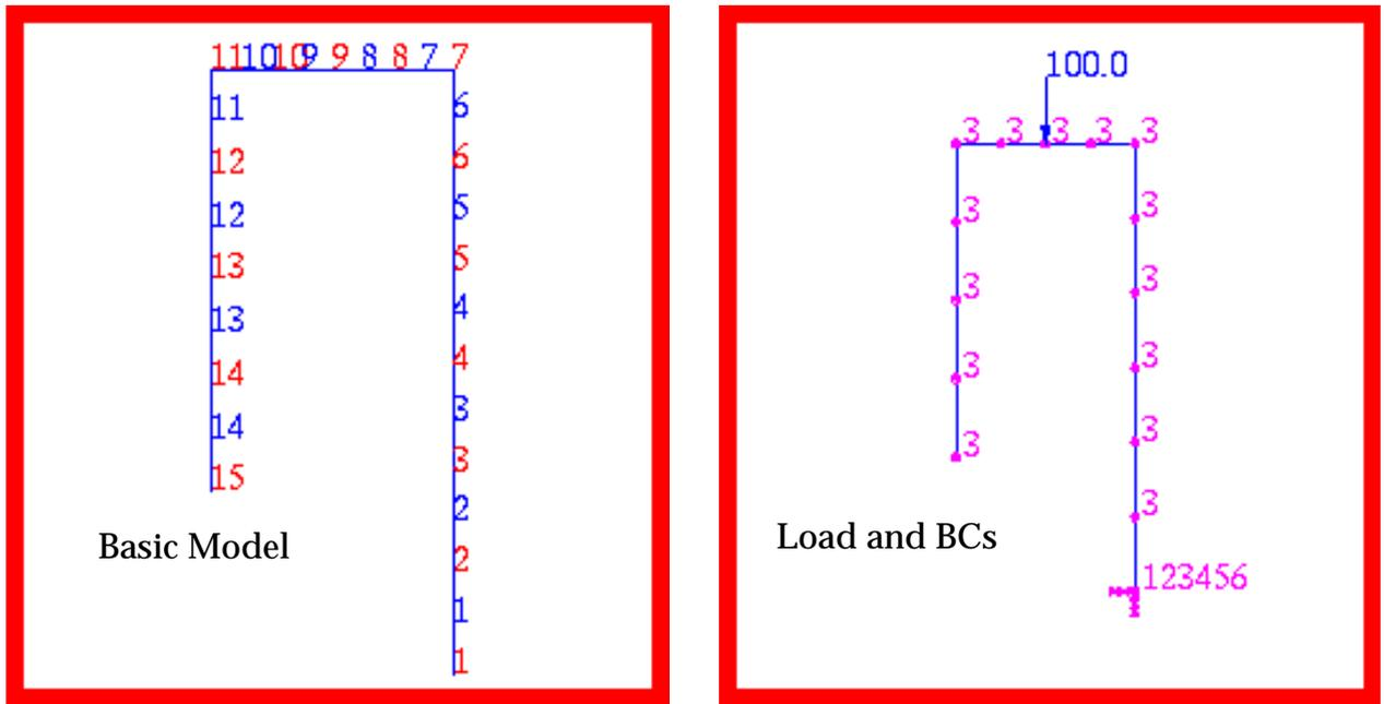
Figure 15-1 Basic FE Model of Rigid Frame with Load and BCs.
