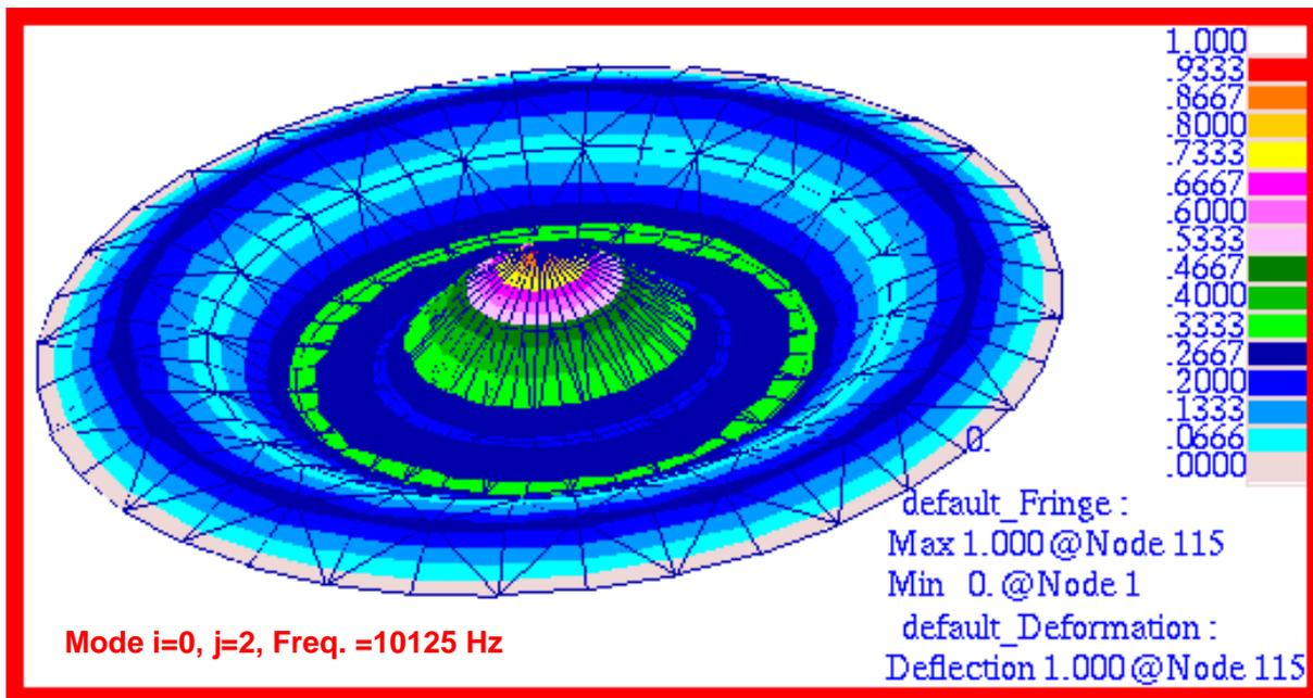
Figure 15-14 Mode 15,  $f_{02}$ , for Membrane h-Element Model.
