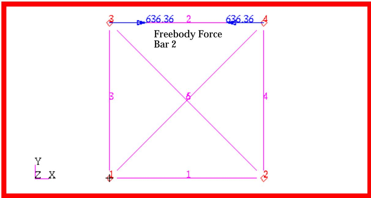
Figure 15-68 Freebody Forces in Bar 2.
