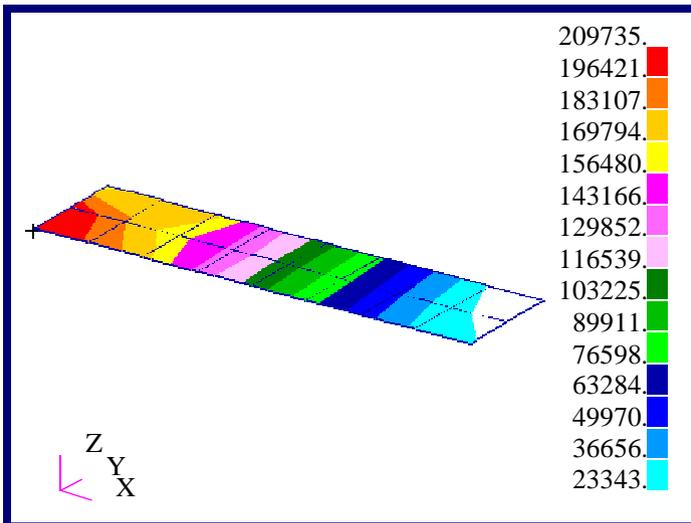
**Figure 4-1 Fringe Plot of von Mises Stress on Cantilever Plate.**
