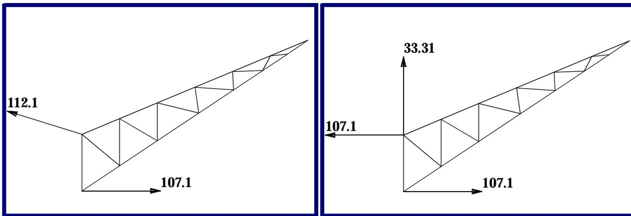
**Figure 12-2 Example Plot of Reaction Loads at the Wall for the Continuous Truss Example. Both Resultant and Component Displays are Shown.**
