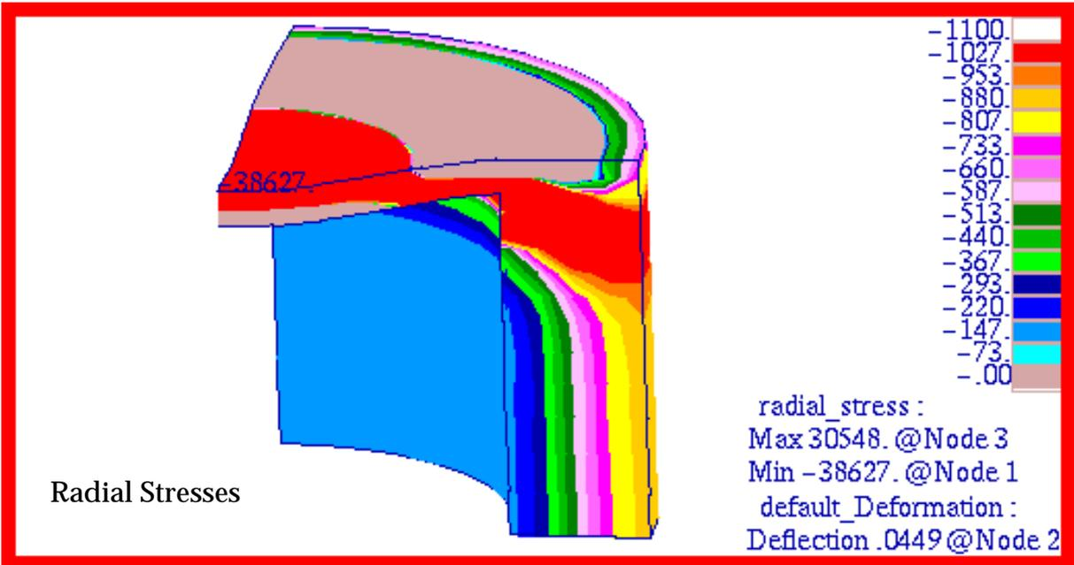
Figure 15-52 Radial,  $\sigma_3$ , Stress of Thick Walled Cylinder.
