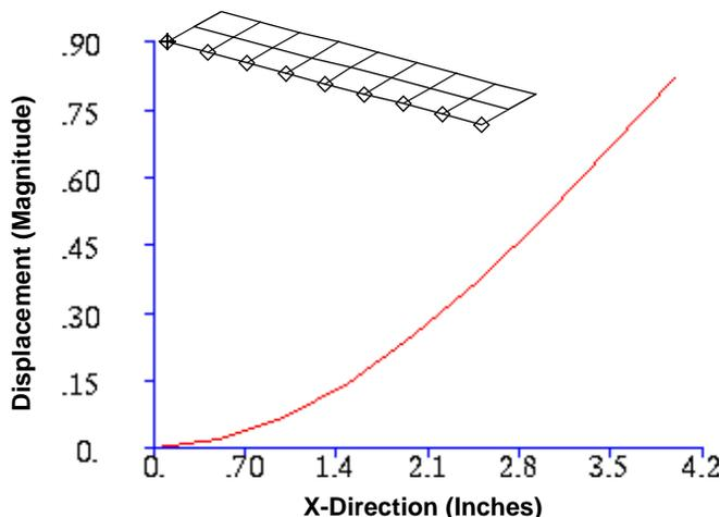
**Figure 8-1 Result Value (Displacement) Versus Distance of the Cantilever Beam's Nodes as Shown.**
