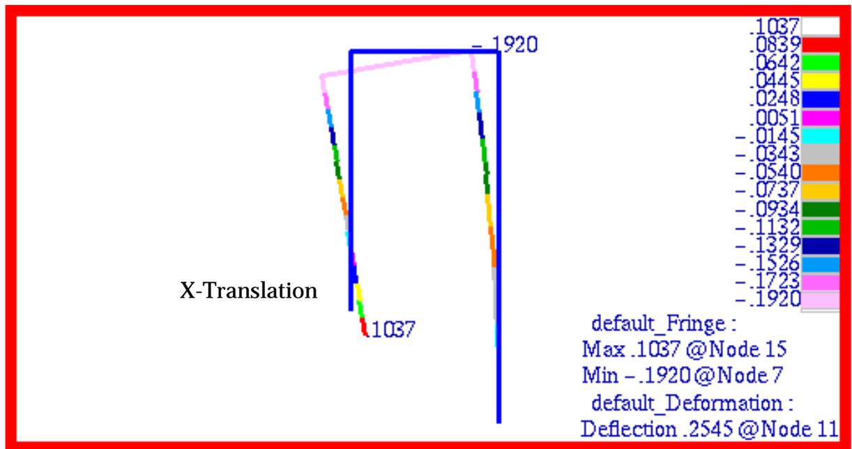
Figure 15-3 X-Translational Deformation of Rigid Frame.
