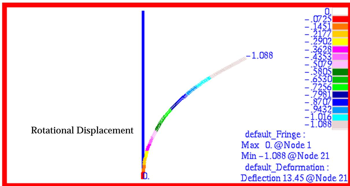
Figure 15-86 Post-Buckled Rotational Deformation about Z of Beam.
