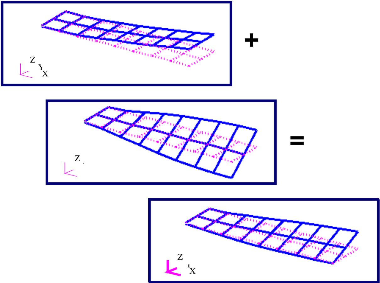
**Figure 11-1 Linear Superposition of Two Load Cases to Create a Third**
