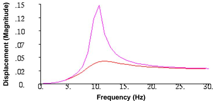
**Figure 8-7 Result Value (Displacement) Versus Global Variable (Frequency) of Different Damping Values.**
