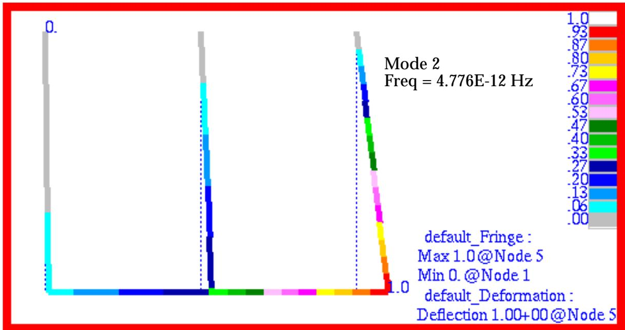
Figure 15-55 Complex Mode 2 of Pendulums, Freq = 4.776E-12 Hz.
