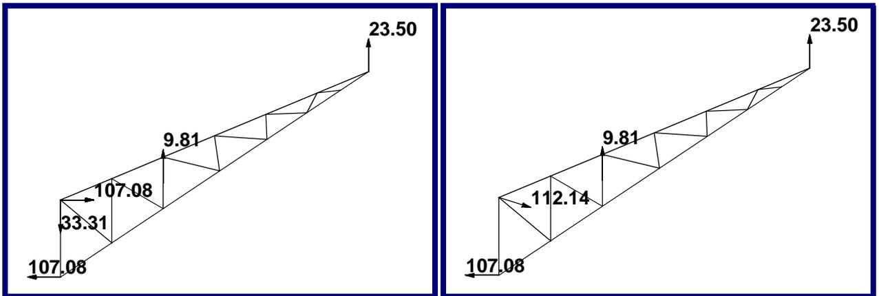
Figure 12-4 Example Plot of Internal Loads for the Continuous Truss Example. Both Resultant and Component Displays are Shown.
