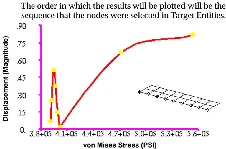
**Figure 8-2 Result Value (Displacement) Versus Result Value (Stress) from the Cantilever Beam's Nodes as Shown.**
