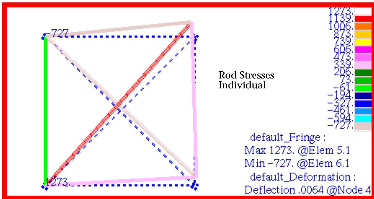
Figure 15-59 Axial Stresses from Pinned Truss Analysis.
