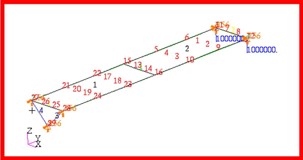
Figure 15-51 p-Element Model of Plate with Suspended Mass.
