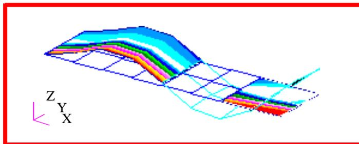
**Figure 4-4 Two Fringe Plots Targeting Certain Elements, One on the Undeformed Shape and One on the Deformed Shape.**
