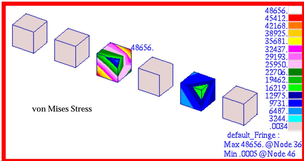
Figure 15-67 von Mises Stress in Elements due to Thermal Gradient.
