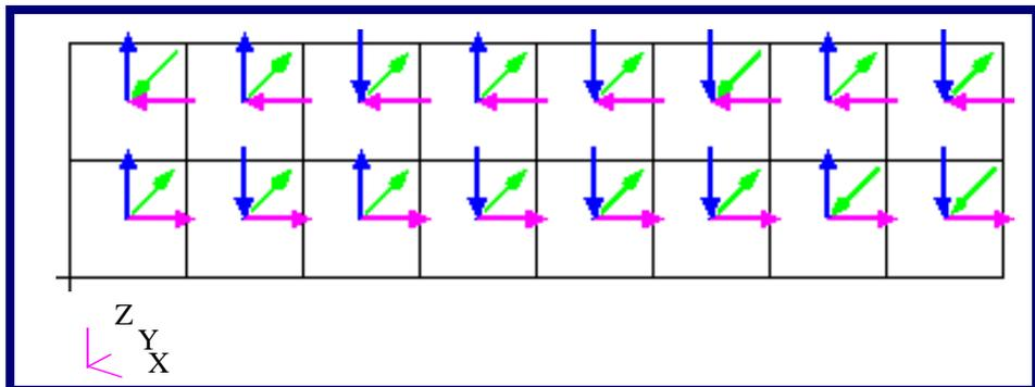
Figure 6-5 A Tensor Plot on the Cantilever Beam Modified to Display in Crow's Feet Form.
