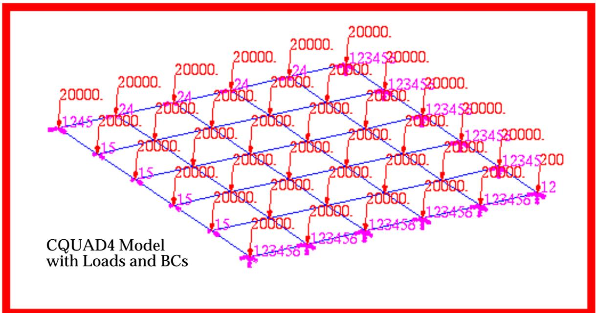
Figure 15-60 CQUAD4 Model of Plate with Loads and BCs.
