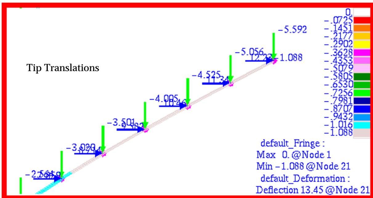
Figure 15-87 Vector Plot of Tip Deflections of Beam.
