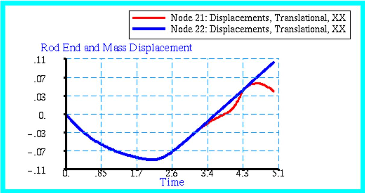
Figure 15-42 Rod End and Mass Displacement Responses.
