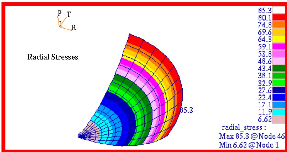
Figure 15-36 Radial Stresses of Spherical Membrane.
