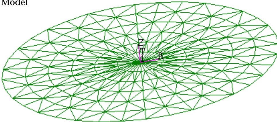
Figure 15-8 Basic Circular Membrane Model with h-Elements.
