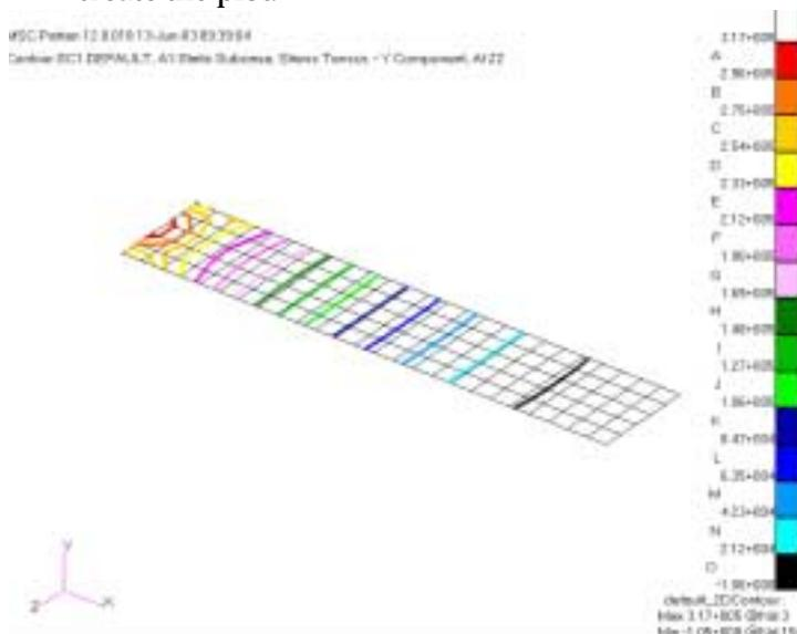
Figure 5-1 Contour Plot of the Y-Component of Stress on Cantilever Plate.
