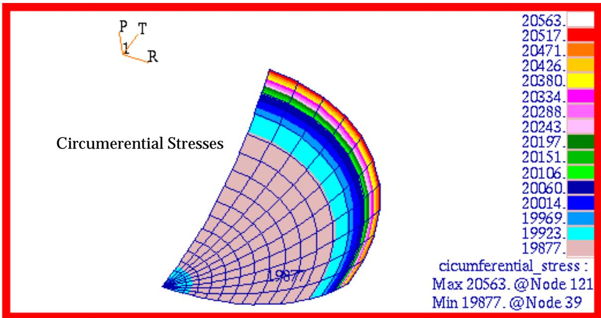
Figure 15-38 Circumerential Stresses of Spherical Membrane.
