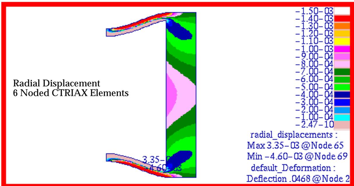
Figure 15-40 Radial Displacement of 6 Noded Axisymmetric Model.
