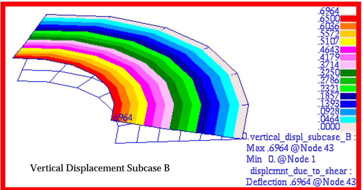
Figure 15-74 Vertical Displacement of Annular Plate (Subcase B).
