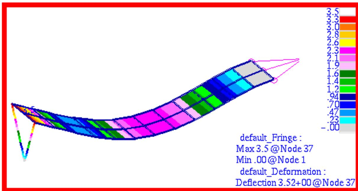
Figure 15-49 Third Mode Shape of Beam, Freq = 71.134 Hz.
