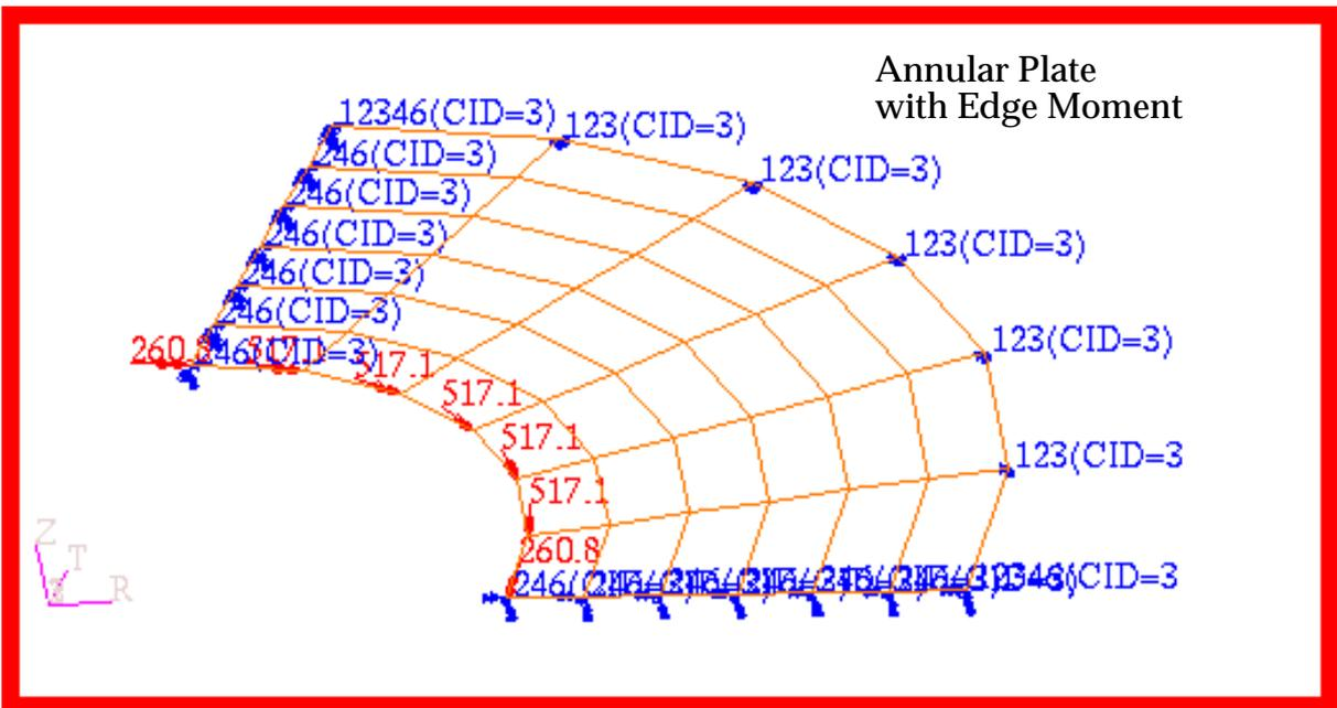
Figure 15-70 Annular Plate with Edge Moment (Subcase C).
