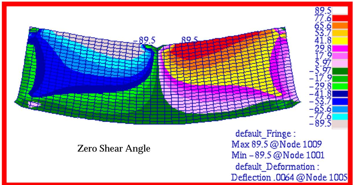
Figure 15-21 Orientation Angle of Maximum Principal Stress.
