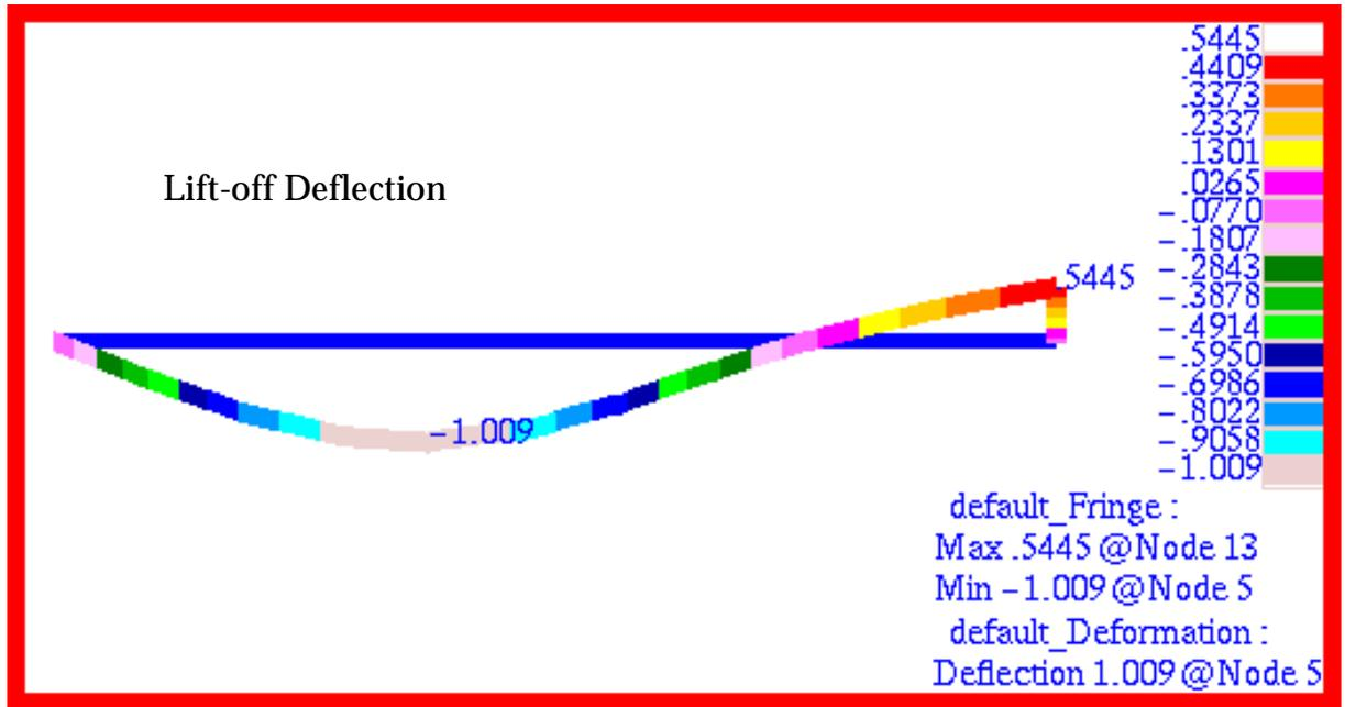
Figure 15-2 Deflection Plot of Lift-off of Beam.
