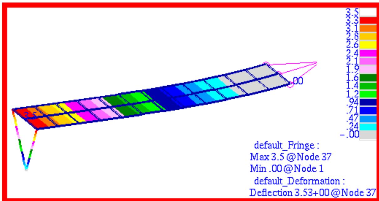
Figure 15-48 Second Mode Shape of Beam, Freq = 12.84 Hz.
