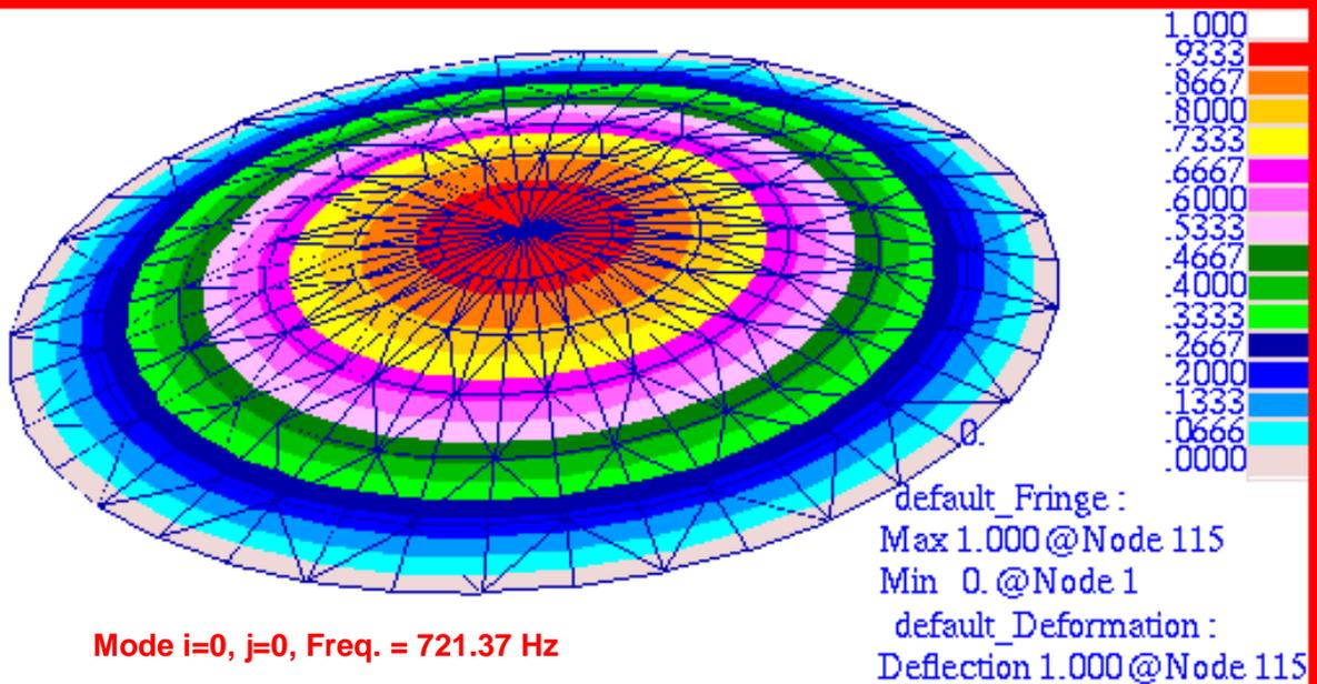
Figure 15-9 Mode 1,  $f_{00}$ , for Membrane h-Element Model.
