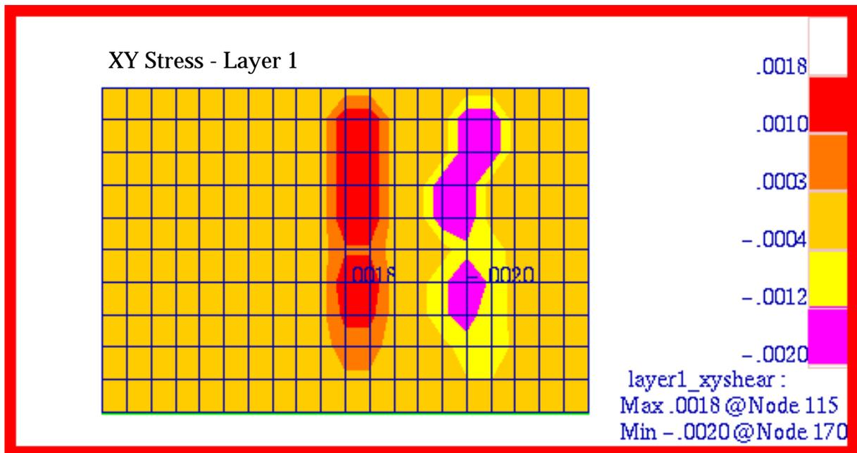
Figure 15-10 Cross-Ply Composite Plate,  $\tau_{xy}$  Stress, Layer 1.
