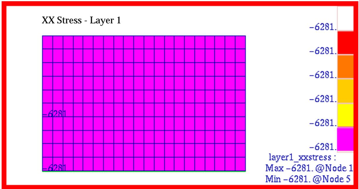
Figure 15-8 Cross-Ply Composite Plate,  $\sigma_x$  Stress, Layer 1.
