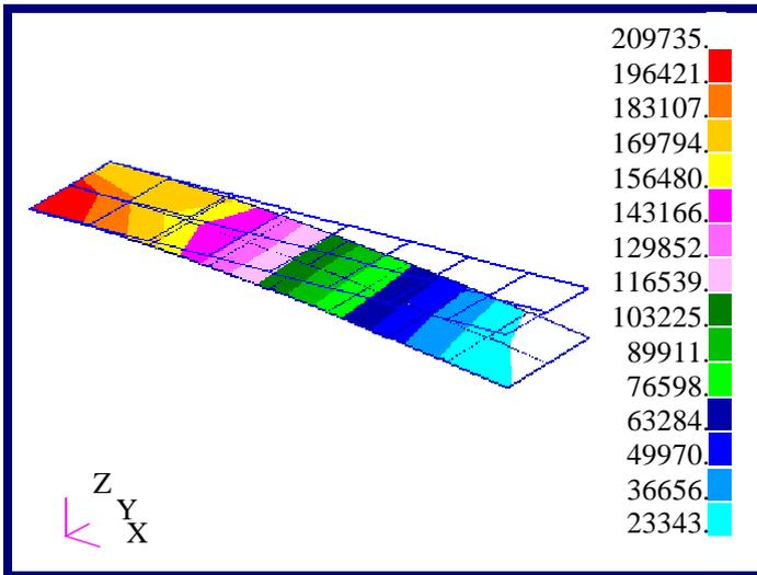
Figure 2-3 Fringe Plot on a Deformation Plot of Cantilever Plate with Undeformed Shape.
