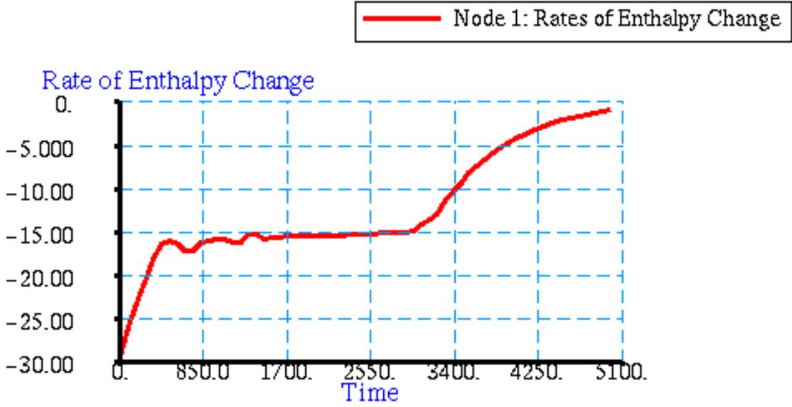
Figure 15-63 Rate of Enthalpy Change of Freezing Cube.
