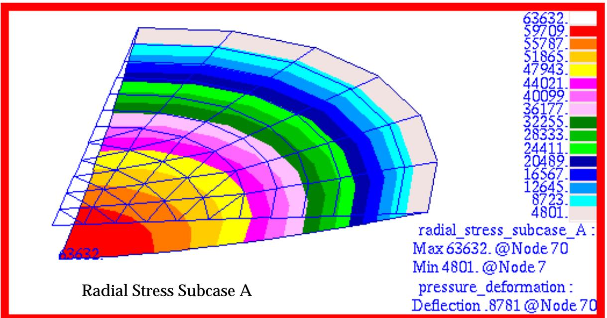
Figure 15-72 Radial Stress of Circular Plate (Subcase A).
