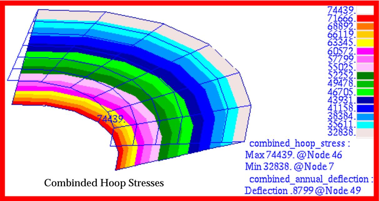
Figure 15-82 Combined Hoop Stress of Annular Plate.
