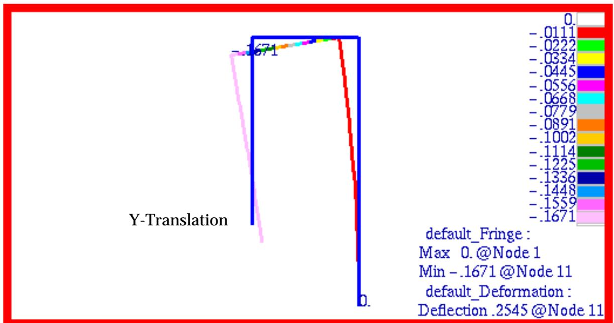
Figure 15-4 Y-Translational Deformation of Rigid Frame.
