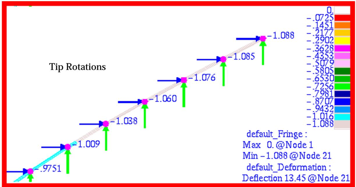
Figure 15-88 Vector Plot of Rotational Deformation of Beam.
