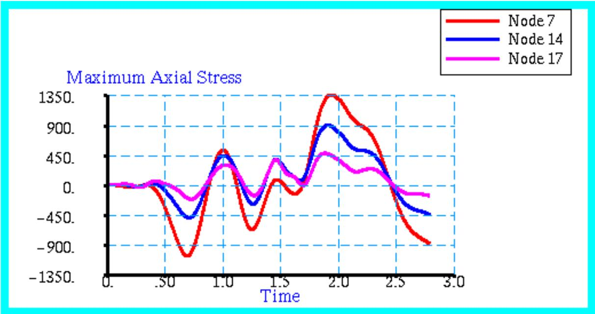
Figure 15-35 Stress Responses at Selected Points in 2D-Truss.
