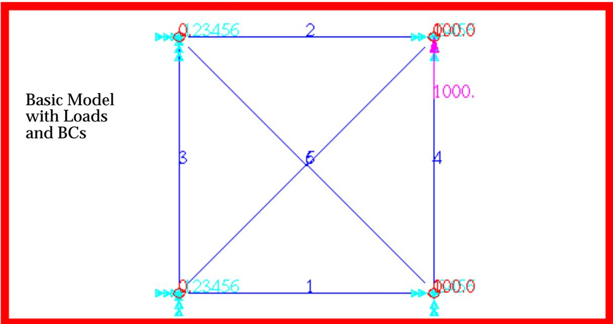
Figure 15-66 Model of Pinned Truss.
