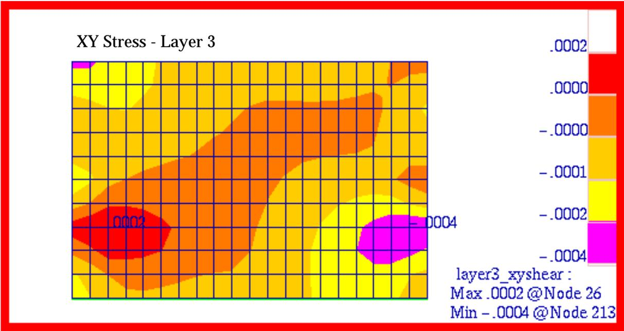
Figure 15-16 Cross-Ply Composite Plate,  $\tau_{xy}$  Stress, Layer3.
