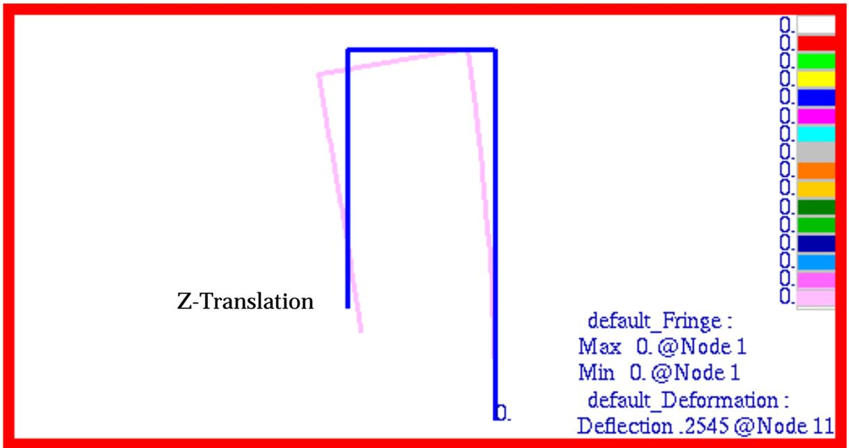
Figure 15-5 Z-Translational Deformation of Rigid Frame.
