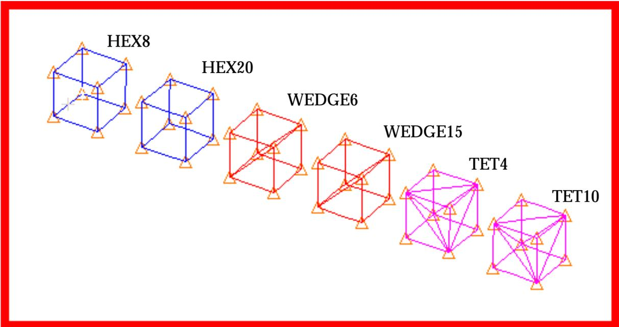
Figure 15-64 Models of Different Solid Element Types.
