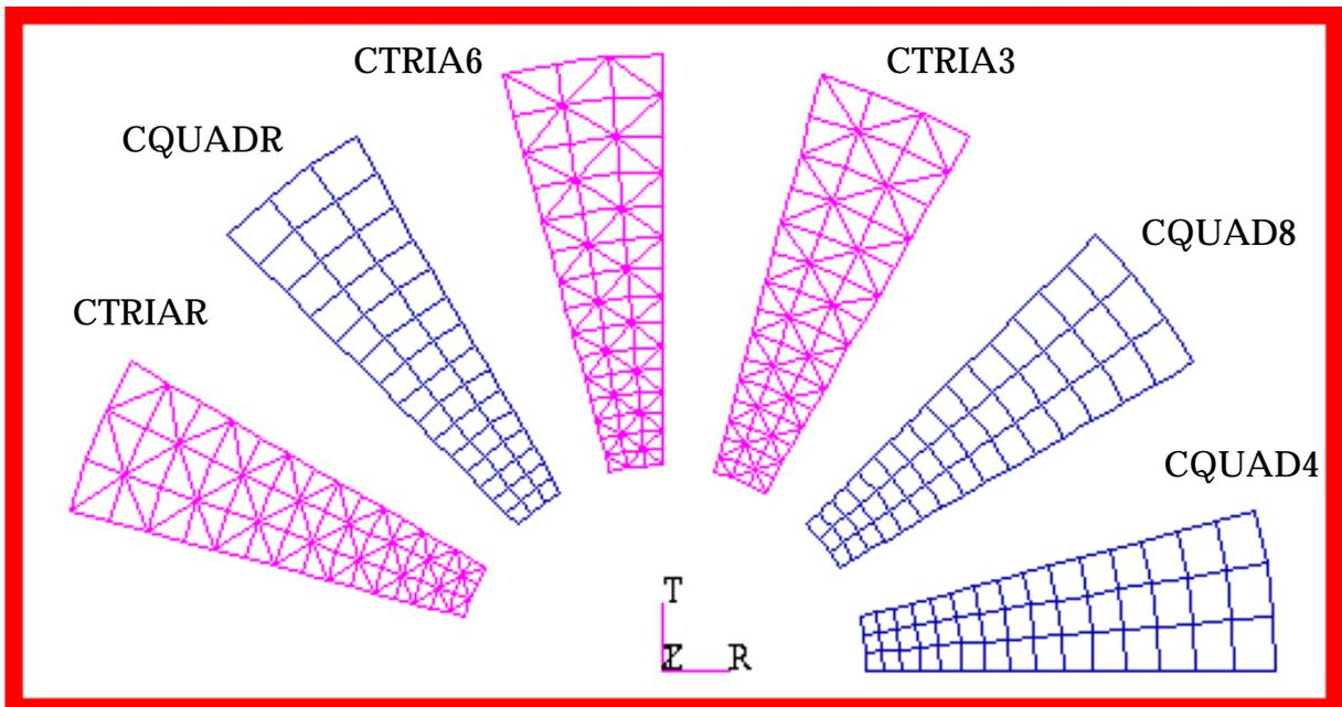
Figure 15-27 Basic Models Using 2D Solid Elements.
