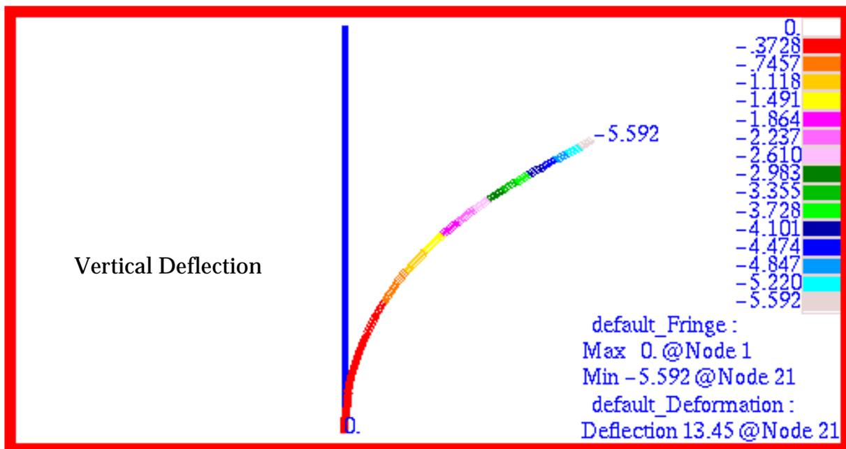
Figure 15-85 Post-Buckled Vertical Deformation of Beam.
