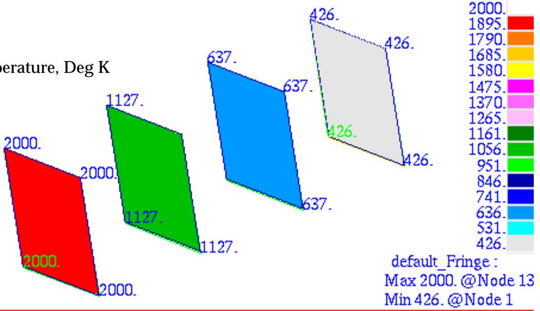
Figure 15-59 Steady State Temperatures of the Four Parallel Plates.
