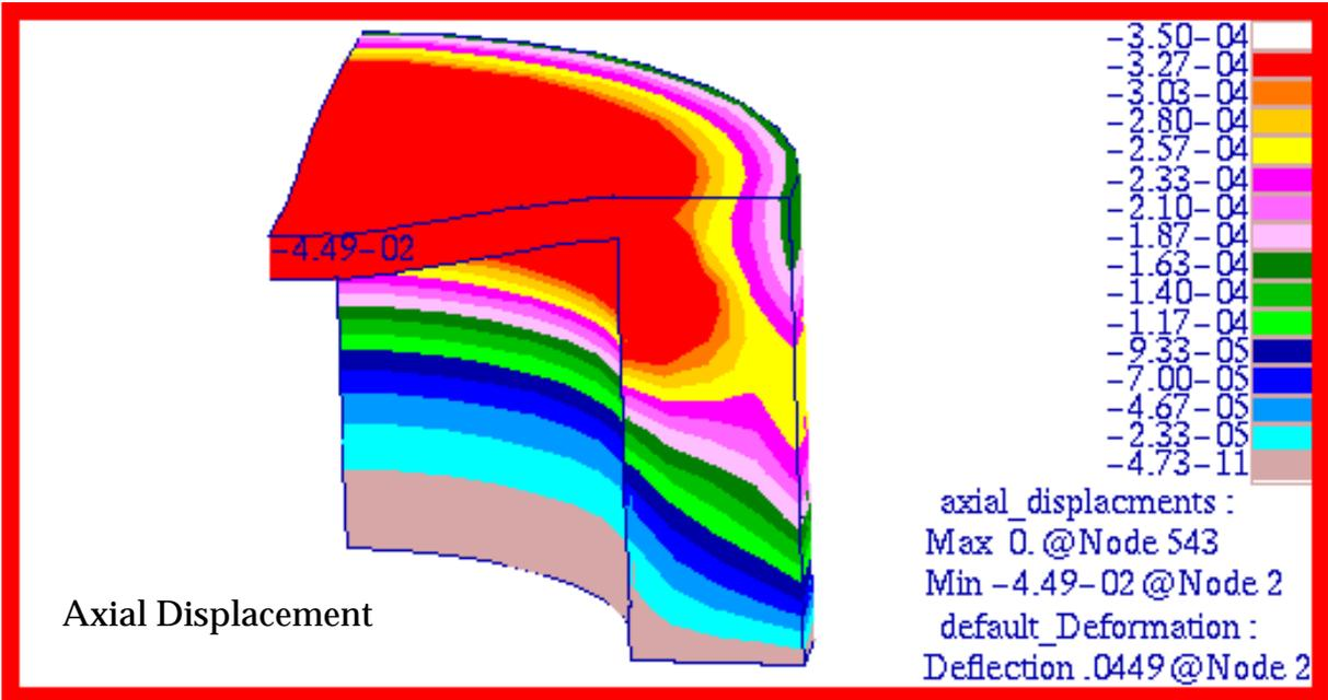
Figure 15-51 Axial Displacement of Thick Walled Cylinder.
