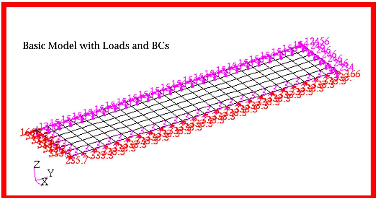
**Figure 15-24 Plate Buckling Model with Load and BCs.**
