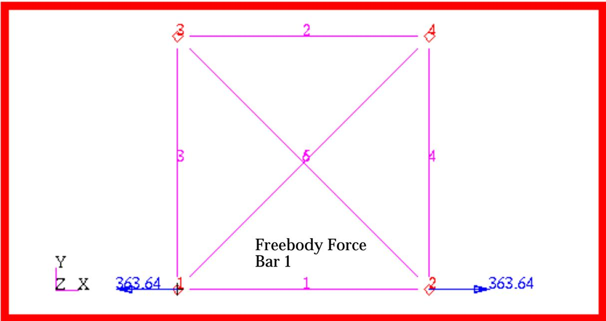
Figure 15-67 Freebody Forces in Bar 1.
