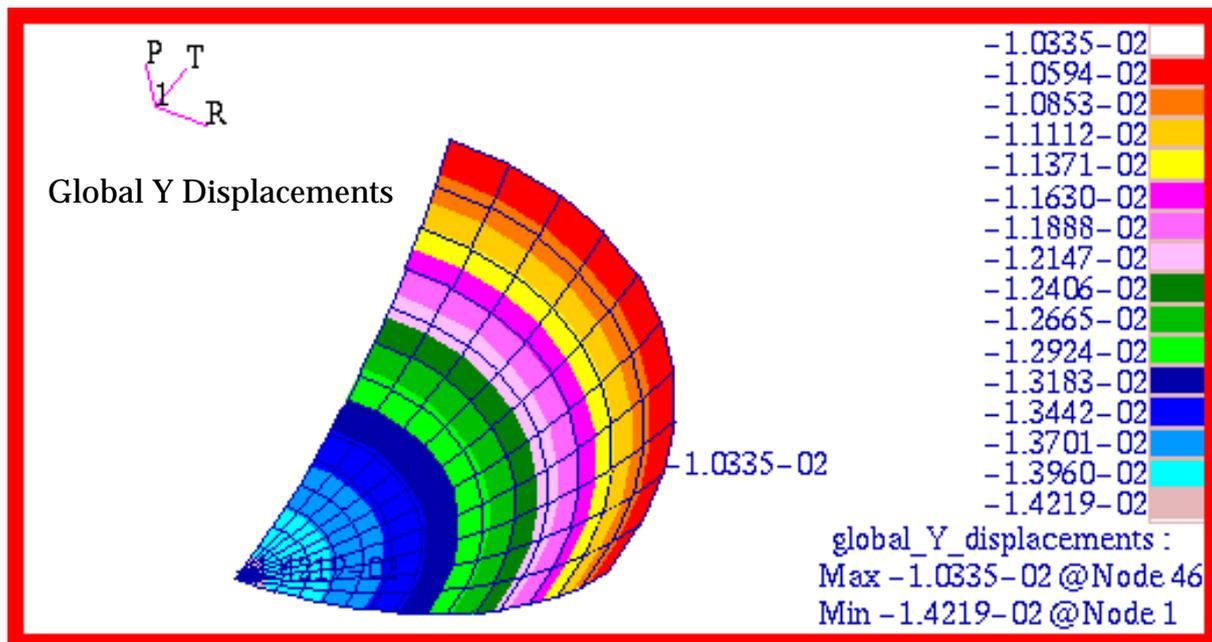
Figure 15-35 Global Translational Y Displacement of Membrane.
