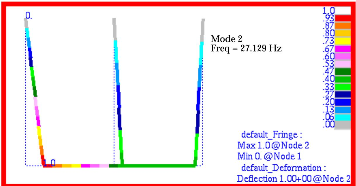
Figure 15-56 Complex Mode 3 of Pendulums, Freq = 27.129 Hz.
