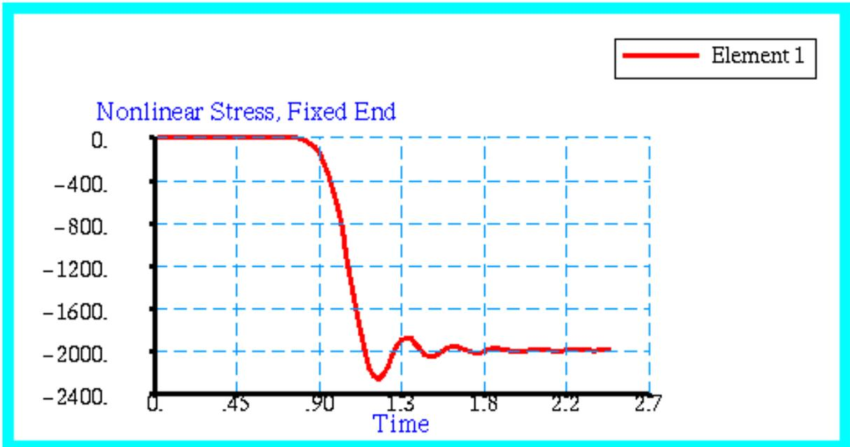
Figure 15-38 Stress History Plot at Element 1, the Fixed End.
