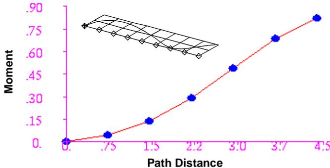
**Figure 8-6 Result Value (Displacement) Along an Arbitrary Path (Defined by a Curve) as Shown on the Cantilever Beam.**
