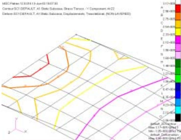
**Figure 5-3 Contour Plot of the Y-Component of Stress on Deformed Cantilever Plate.**
