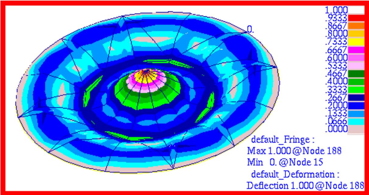
Figure 15-21 Mode 15,  $f_{02}$ , of p-Element Membrane Model.
