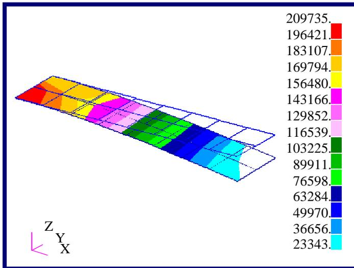
**Figure 3-3 Fringe Plot on a Deformation Plot of Cantilever Plate with Undeformed Shape.**
