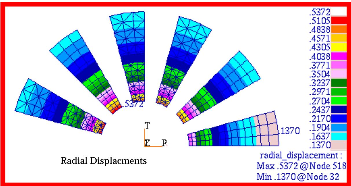
Figure 15-29 Fringe Plot of Radial Displacement on 2D Solids.
