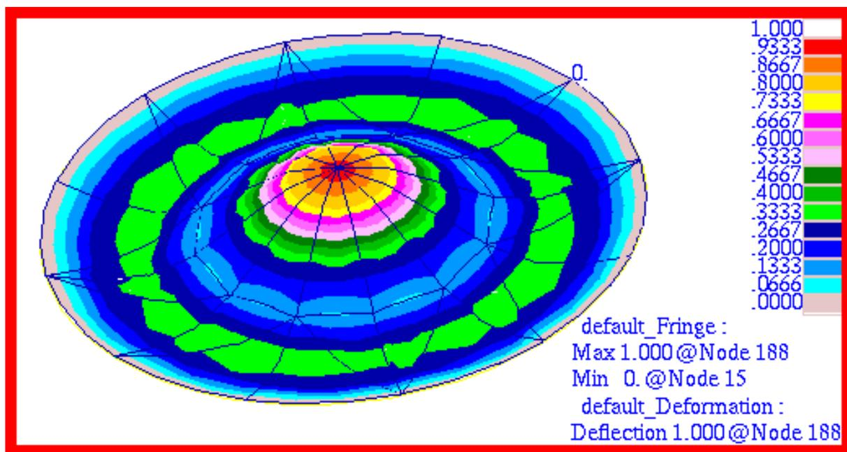
Figure 15-19 Mode 6,  $f_{01}$ , of p-Element Membrane Model.
