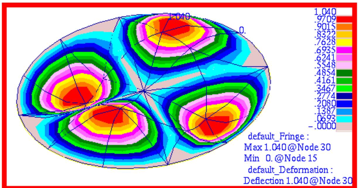
Figure 15-18 Mode 4,  $f_{20}$ , of p-Element Membrane Model.
