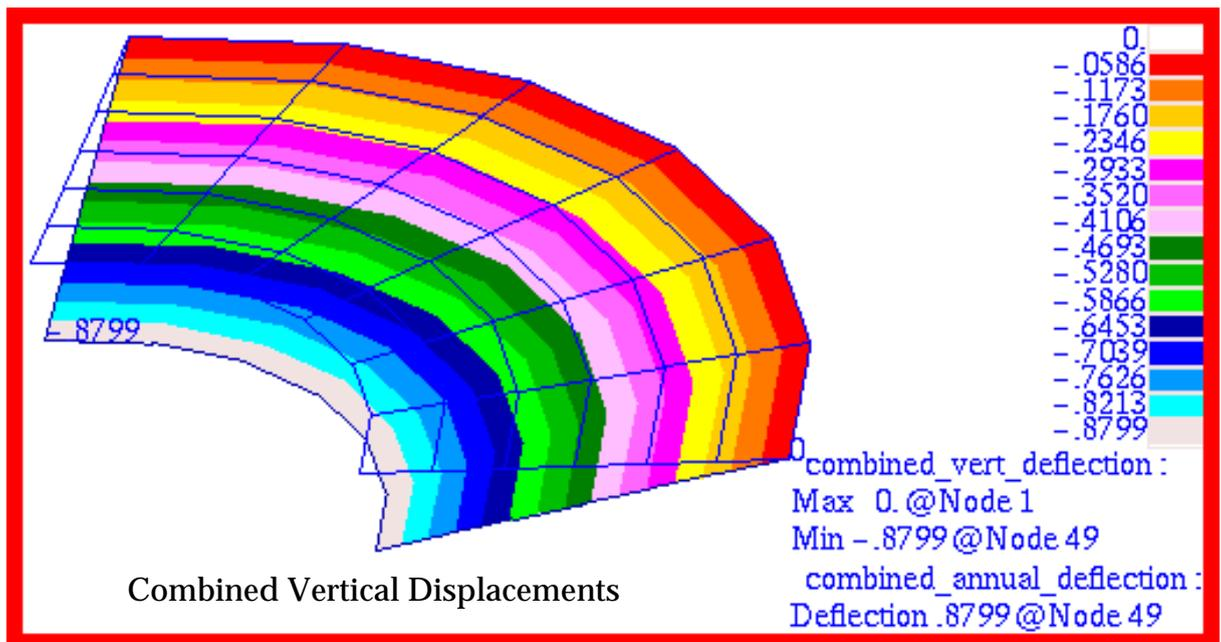
Figure 15-80 Combined Vertical Displacements of Annular Plate.
