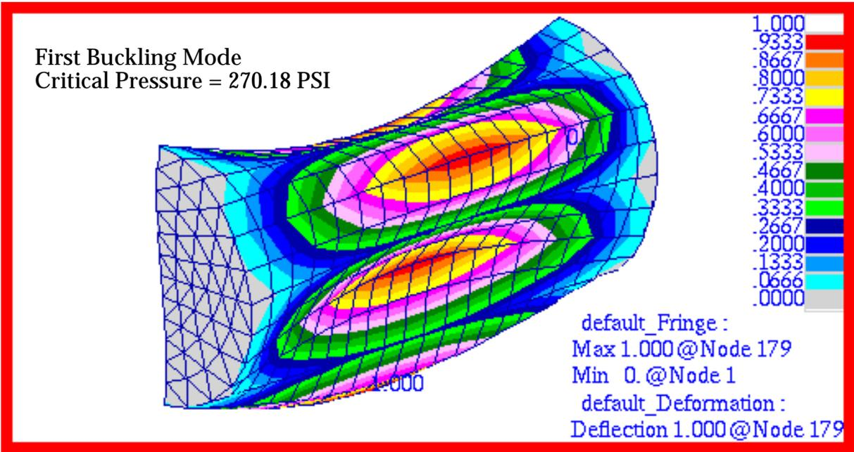
Figure 15-23 Three Lobed Mode Corresponding to Critical Pressure.
