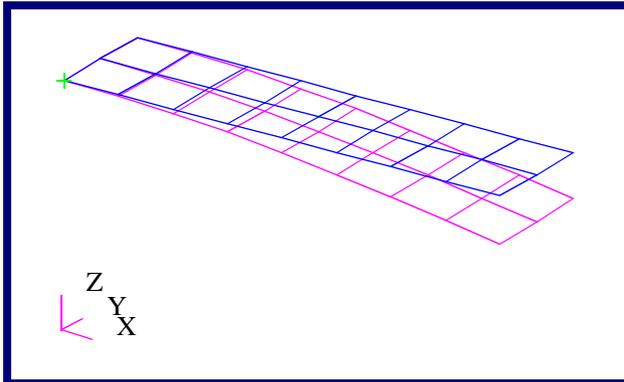
**Figure 2-2 Deformation Plot of Cantilever Plate with Undeformed Shape.**
