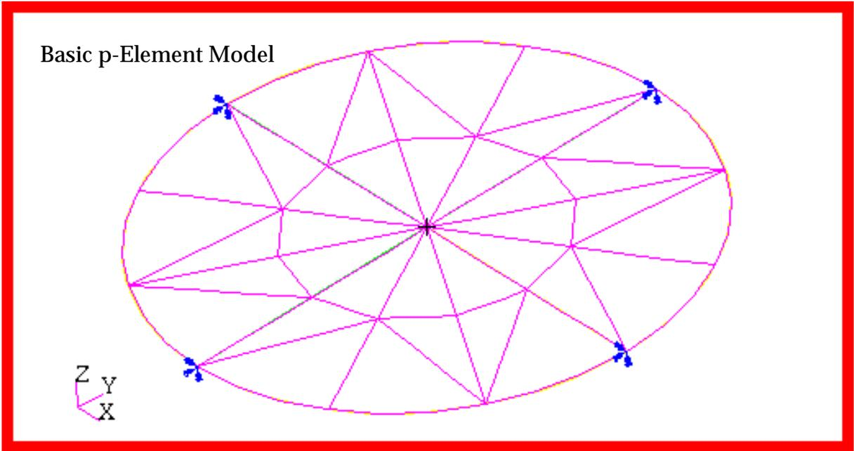
Figure 15-15 Basic p-Element Membrane Model.
