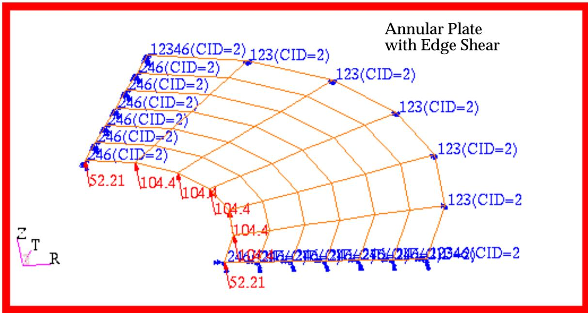
Figure 15-69 Annular Plate with Edge Shear (Subcase B).
