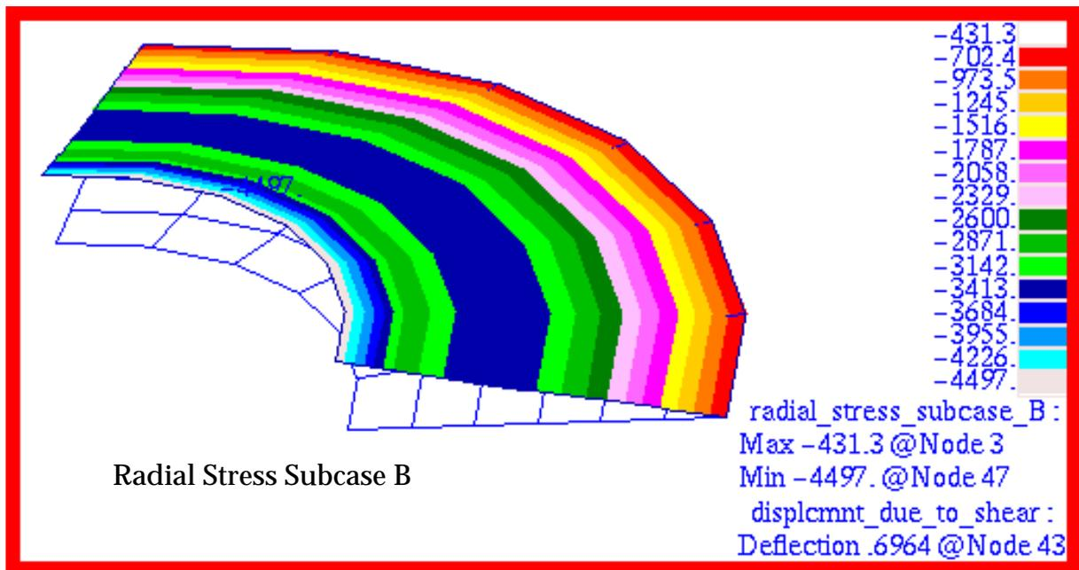
Figure 15-75 Radial Stress of Annular Plate (Subcase B).
