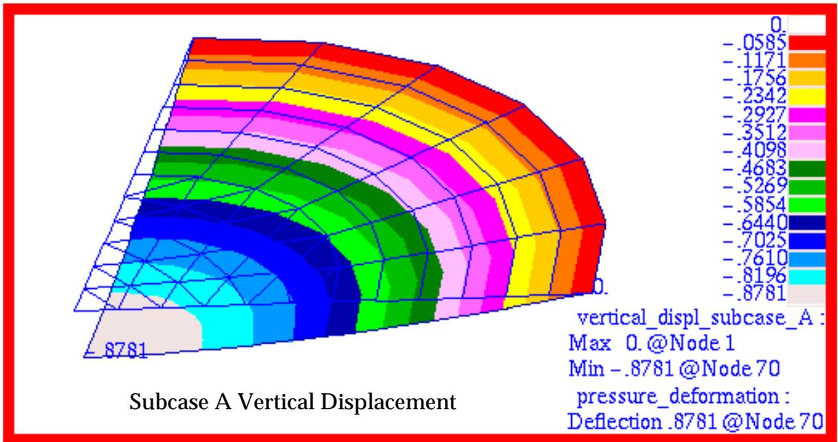
Figure 15-71 Vertical Displacement of Circular Plate (Subcase A).
