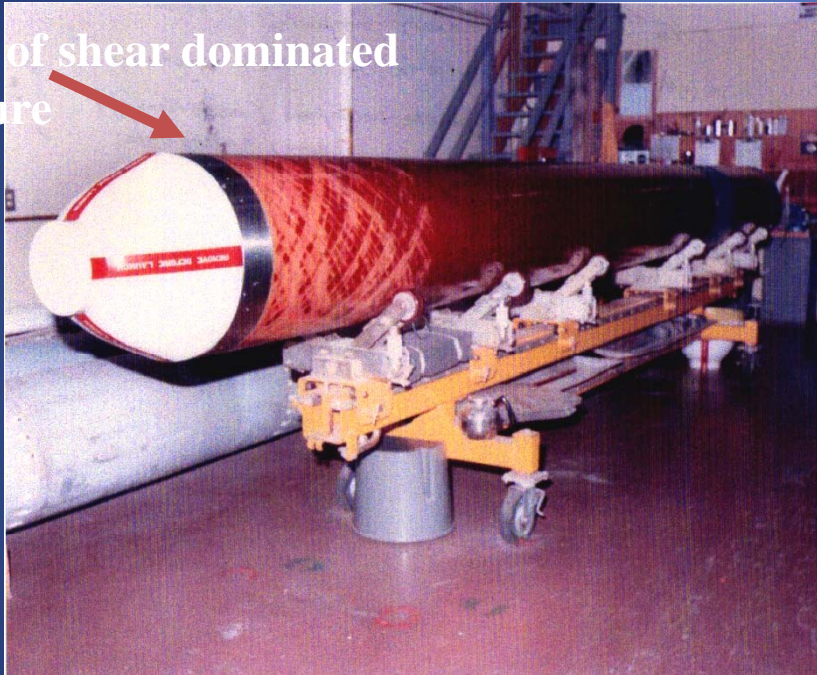
Lightweight Tomahawk Missile Capsule Steel/S-Glass Composite Joint
