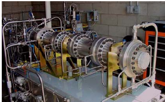
20 MWt CES Gas Generator: Combuster section and 4 sequential water-cooldown sections.
