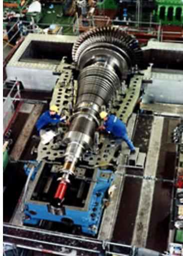
Siemens N-type turbines are used for normal to medium live steam conditions (100 bars, 500 °C). This type of turbine has a reaction-type design that has proven itself many times over. N-type turbines can be either **condensing** or **backpressure** machines. The standard configuration allows up to two controlled **extractions** and/or several uncontrolled extraction points.
