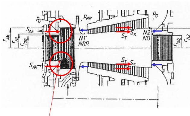
Balance piston allows balancing of axial forces
