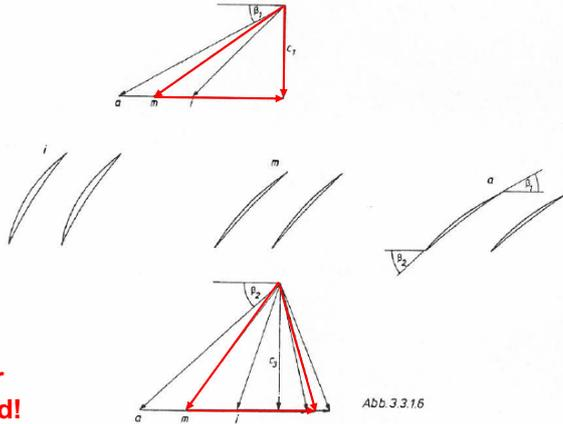
**Rotor and stator blade are twisted!**
