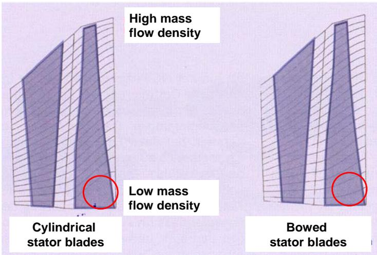
The diagram compares the meridional streamlines for two types of stator blades:
