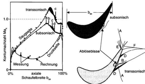
Mach number distribution along suction and pressure side of a turbine at subsonic and transonic conditions
