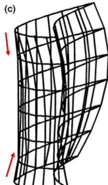
**Figure 6.11.** Section stacking: (a) radial stack (b) and (c) 3D stacks.
