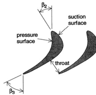
**Figure 6.5.** Turbine stage: principal objectives.
