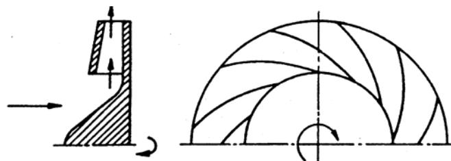
Linear cascade of a radial machine
