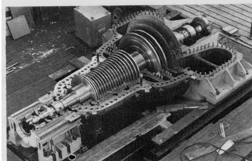
20/25 MW Extraction-Condensation turbine, live steam 70 bar, 525°C, extraction pressure 2,6 bar, Condensation pressure 0,032 bar
