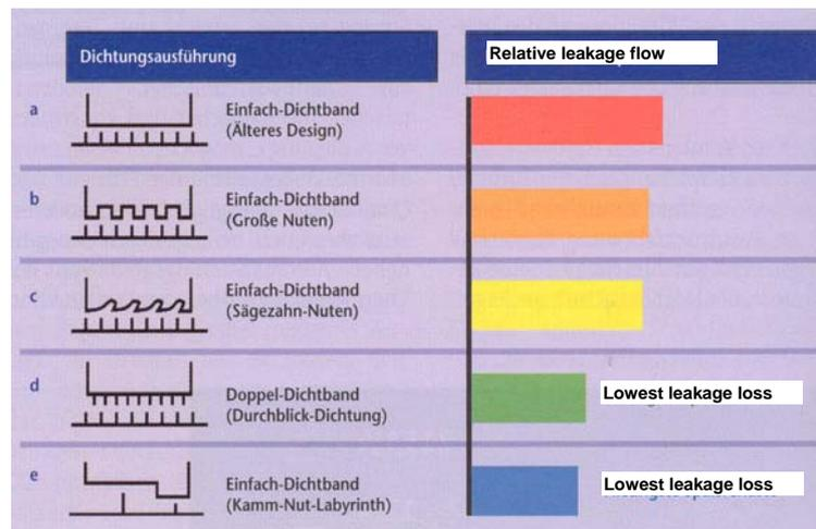
Flow through sealings is a repeated throttle flow
