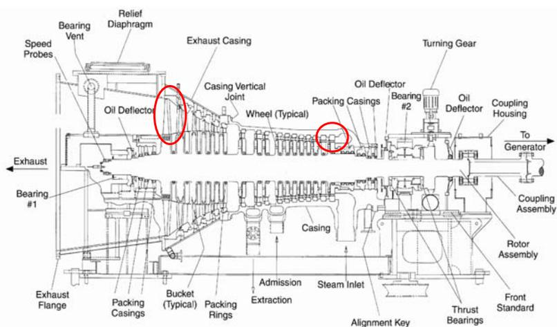
Figure 6. Nonreheat, single-casing, axial exhaust steam turbine
