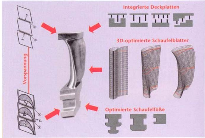
The diagram illustrates the components of modern 3D blade geometry. A central 3D model of a blade is shown with red arrows pointing to four categories of components:
