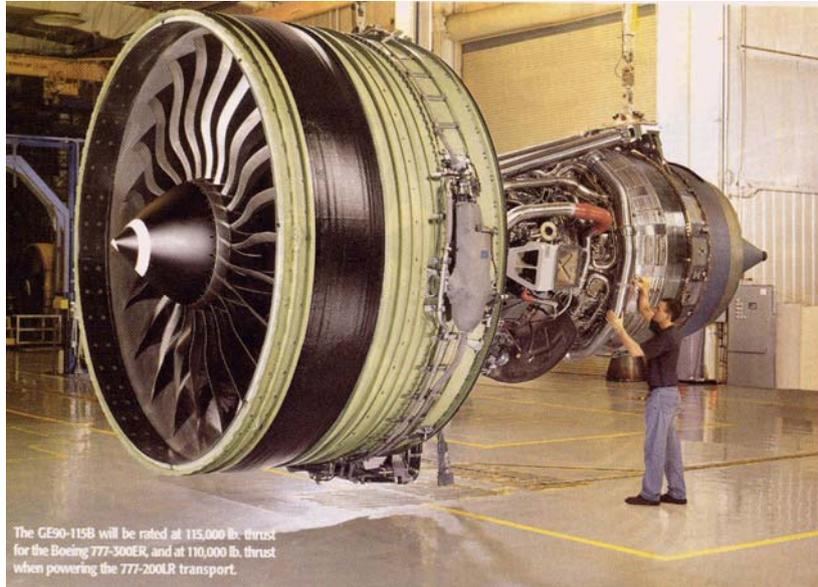
The GE90-115B will be rated at 115,000 lb. thrust for the Boeing 777-300ER, and at 110,000 lb. thrust when powering the 777-200LR transport.
