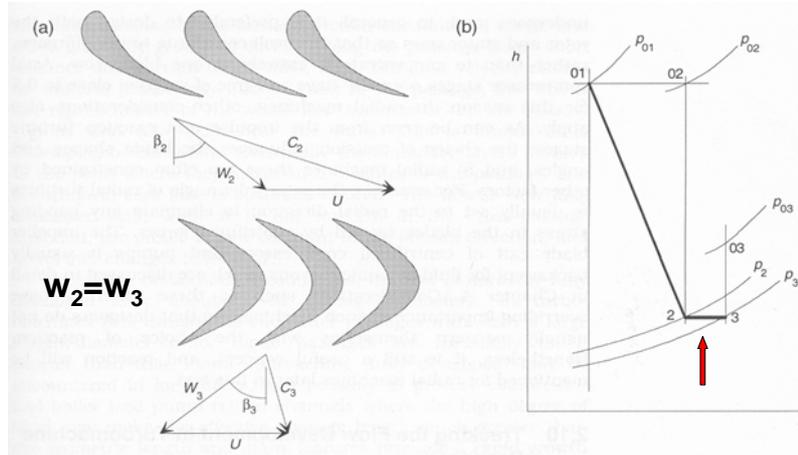
Figure 2.20. Impulse turbine (a) Schematic diagram (b) Mollier diagram.
